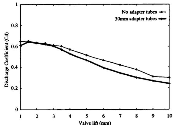
Figure 6 Discharge coefficient comparison for no tubes and 30 mm tubes inserted.
