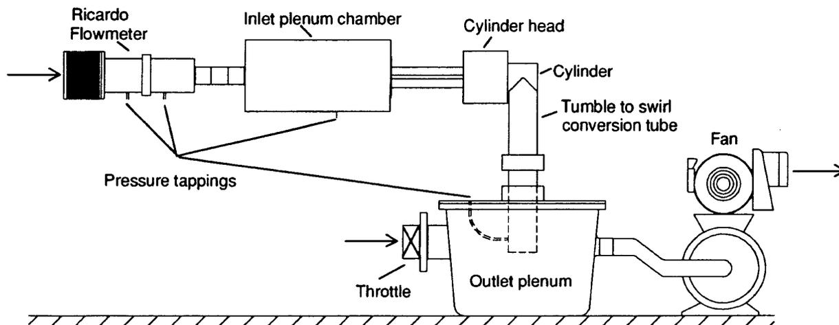
Figure 3 Schematic diagram of steady state air flow rig
