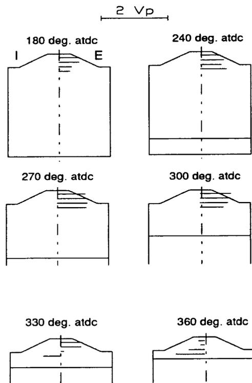
Figure 9a Velocity vector diagrams- no tubes inserted
