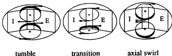
Figure 10 Illustration of barrel swirl breaking down into two counter rotating horizontal vortices
