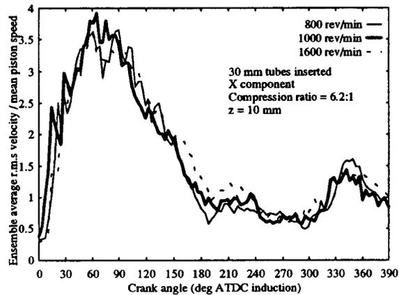
Figure 7b Effect of engine speed on r.m.s velocities
