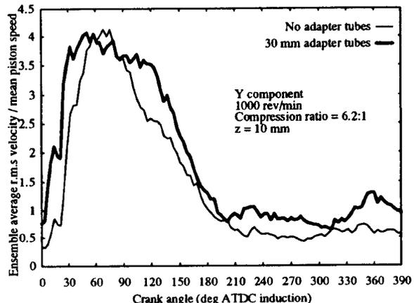
Figure 11b Effect of modified ports on ensemble r.m.s velocities - Y component.
