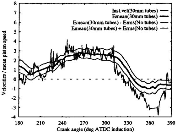
Figure 12a Four consecutive engine cycles - no tubes inserted, 1000 rev/min, 6.2:1, z = 10 mm
