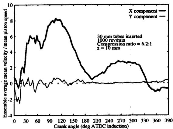
Figure 8b Comparison of mean X and Y components Pent roof chamber - 30 mm tubes inserted
