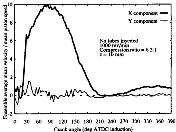
Figure 8a Comparison of mean X and Y components Pent roof chamber - no tubes inserted.
