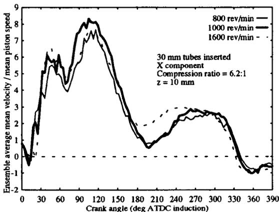
Figure 7a Effect of engine speed on mean velocities
