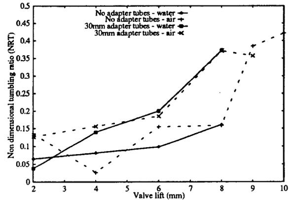
Figure 5 Non Dimensional rig tumble comparison for no tubes and 30 mm tubes inserted.
