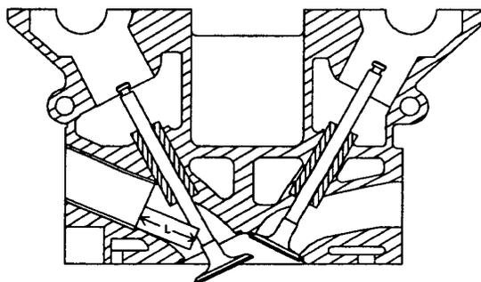
Figure 2 Four-valve cylinder head with pent roof chamber - Section A-A, showing tubes of length L
