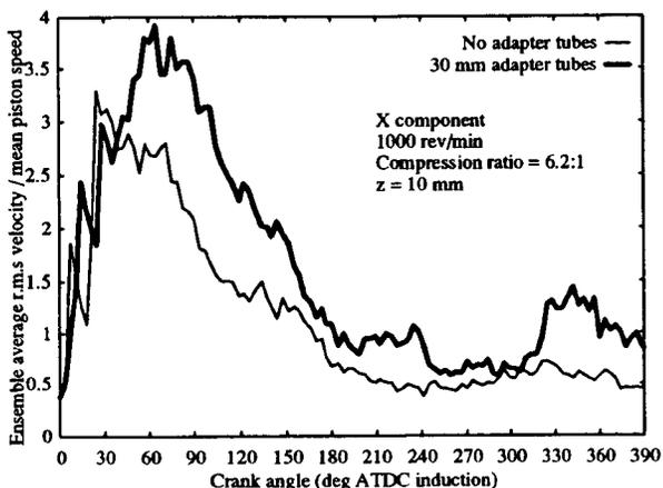
Figure 11a Effect of modified ports on ensemble r.m.s velocities - X component.
