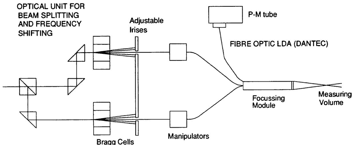
Figure 4 Schematic diagram of fibre-optic Laser Doppler Anemometer
