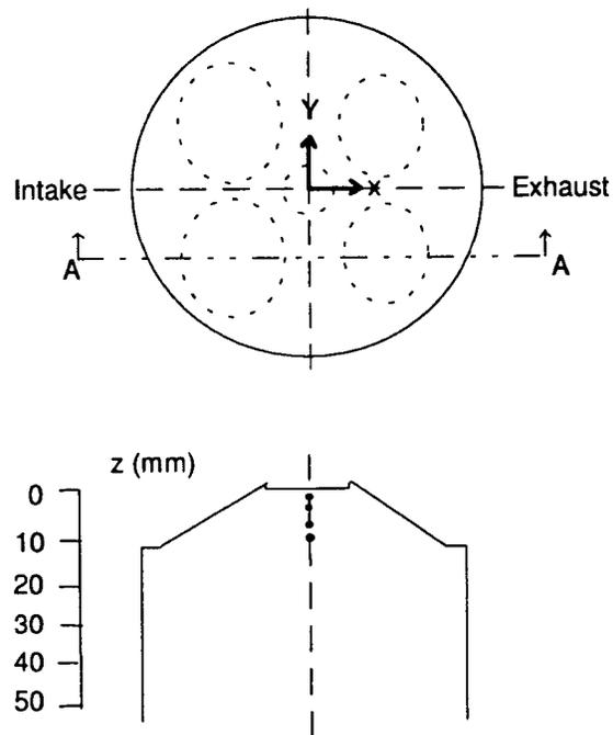
**Figure 1 Four-valve pent roof chamber showing velocity components and sign conventions.**
