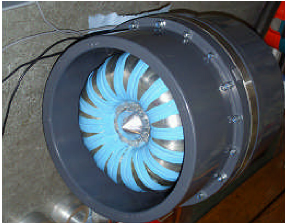
Fig. 14. Tested prototype of the double Halbach array alternator.
