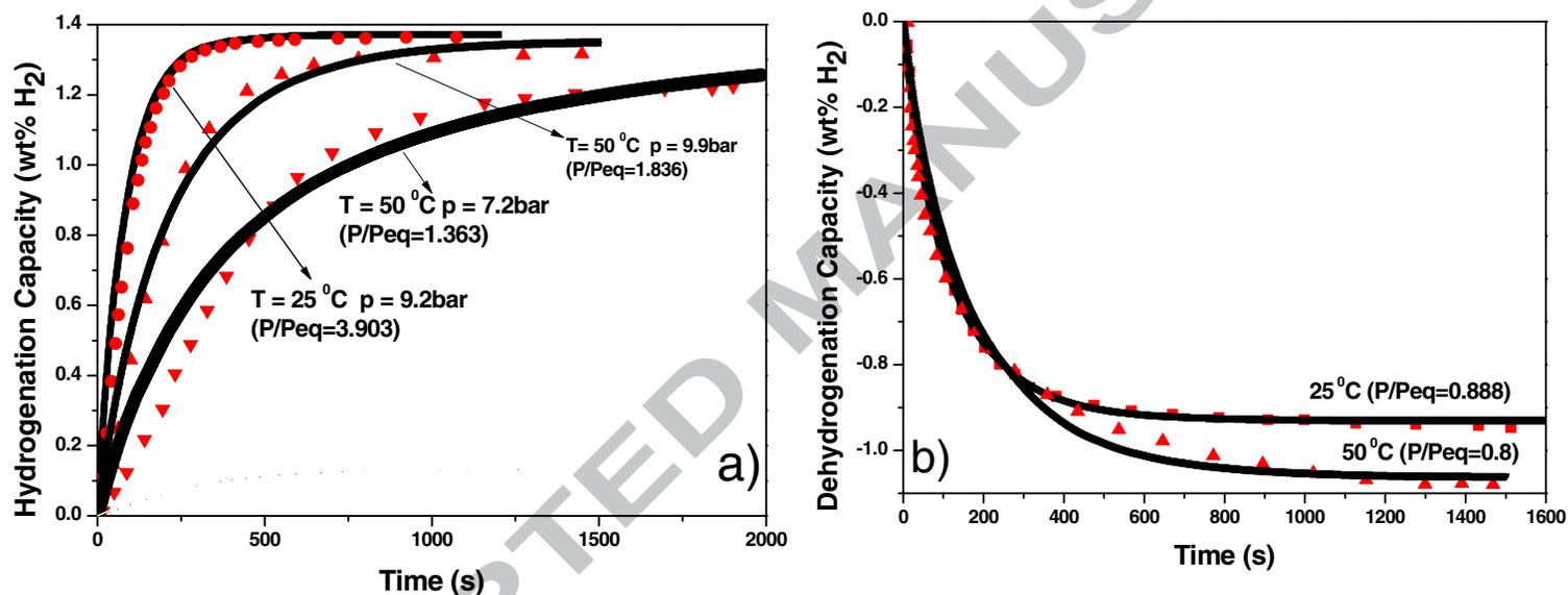
Fig.3. Validation of the predicted amount of hydrogen stored (3a) for different temperatures and different pressures and released (3b) for two different temperatures with experimental data extracted from a lab scale Sievert type apparatus. The experimental results (red dots) with the simulation results (black lines) are in good agreement with a maximum deviation less than 5%.
