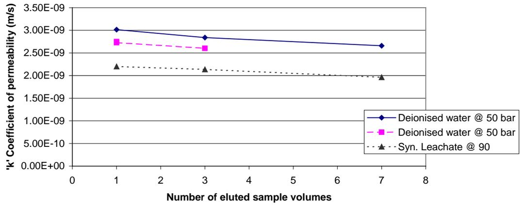
Fig. 5: Permeability Vs. eluted sample volume for 15 MPa. Cement mortar mix.
