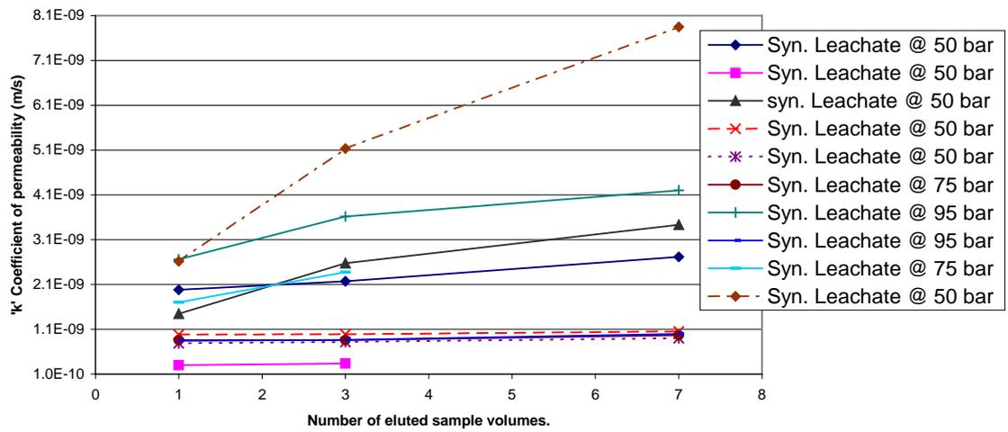
Fig. 6: Permeability Vs. eluted sample volume for 20 MPa. Cement mortar mix.
