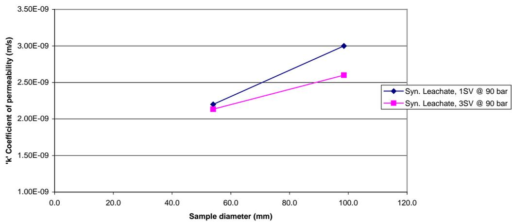
Fig. 8: Coefficient of permeability Vs. Sample size for 15 MPa cement mortar mix.
