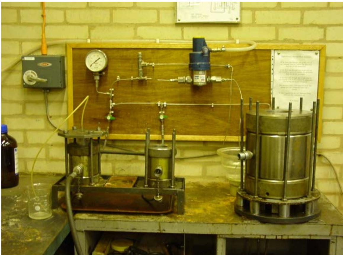
Fig. 3 Modifications to Hoek Cell for Concrete Permeability Measurements
