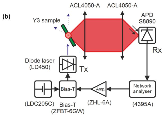
**Figure 3:** a) Result of small signal modulation bandwidth measurement for the Y3 BODIPY. The dotted line corresponds to -3 dB attenuation which defines the bandwidth of the system. b) Experimental setup used for the bandwidth and data transfer measurements.
