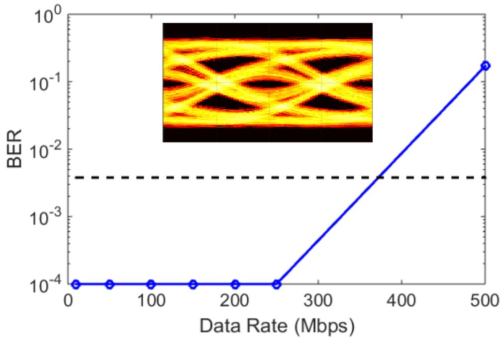
**Figure 4:** Plot of BER versus data rate for OOK. The dashed line corresponds to BER of  $3.8 \times 10^{-3}$  which is defined as the acceptable error floor for VLC. As inset, the eye diagrams at 250 Mb/s are presented.
