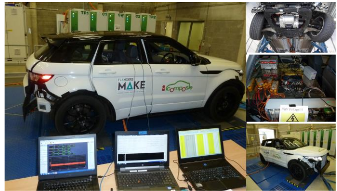
Fig. 3. The Range Rover Evoque set-up on the rolling road facility at Flanders MAKE (Belgium)
