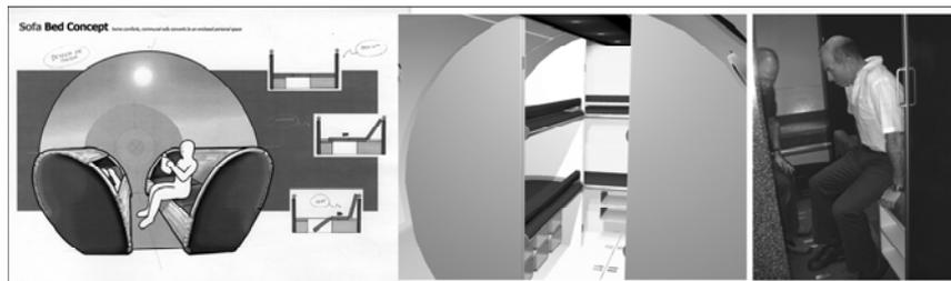
**Figure 1. Sketch concept translation into computer file and mockup evaluation**
