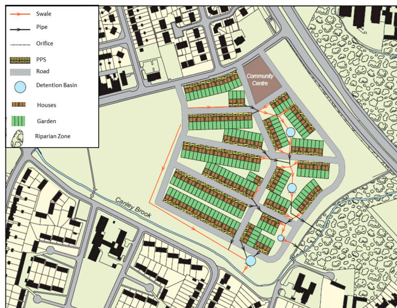
Figure 5. SuDS management train designed for Prior Deram Park, CRZ, Coventry. Site design details are in colour. Some context details derived from Ordnance Survey © Crown Copyright and Database Right 2012. Ordnance Survey (Digimap Licence). Adapted from [14].
