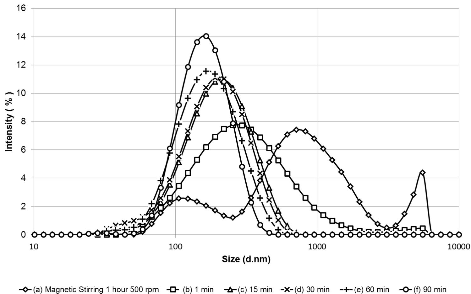
Figure 5. Copper nanoparticle cluster size distribution - intensity plots after 20 kHz ultrasonic probe, 1.3 cm diameter replaceable tip, 100 % amplitude compared with magnetic stirring.
