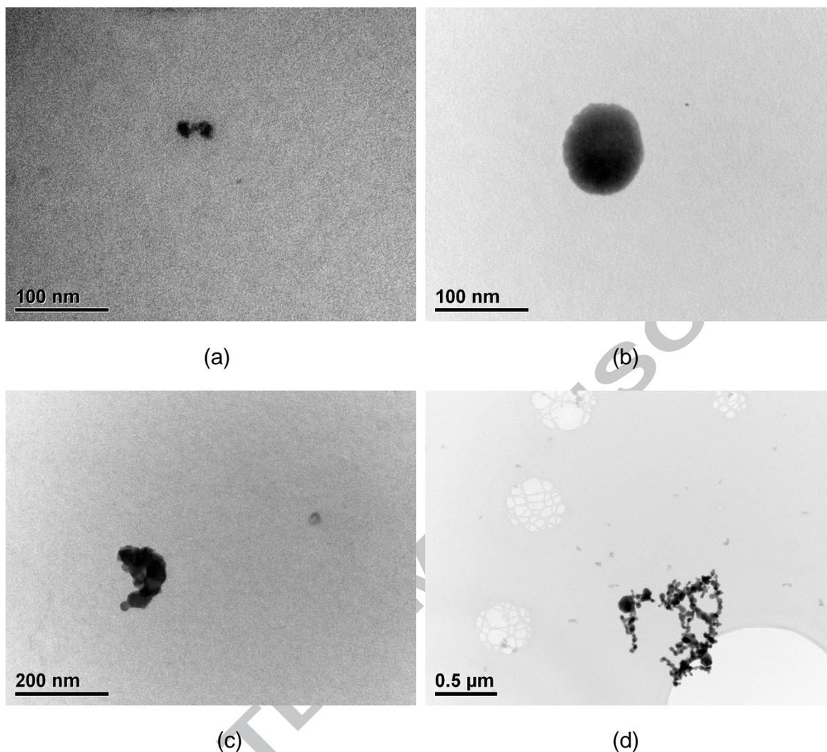
Figure 8. TEM micrographs of copper aggregates after ultrasonic dispersion in propan-2-ol using a 20 kHz ultrasonic probe, 100 % amplitude, 30 min processing time, (a) sub 50 nm (b) sub 100 nm and (c) 25nm and sub 200nm aggregate side by side (d) low magnification image of large aggregates in the foreground and sub 100nm aggregates in the background.
