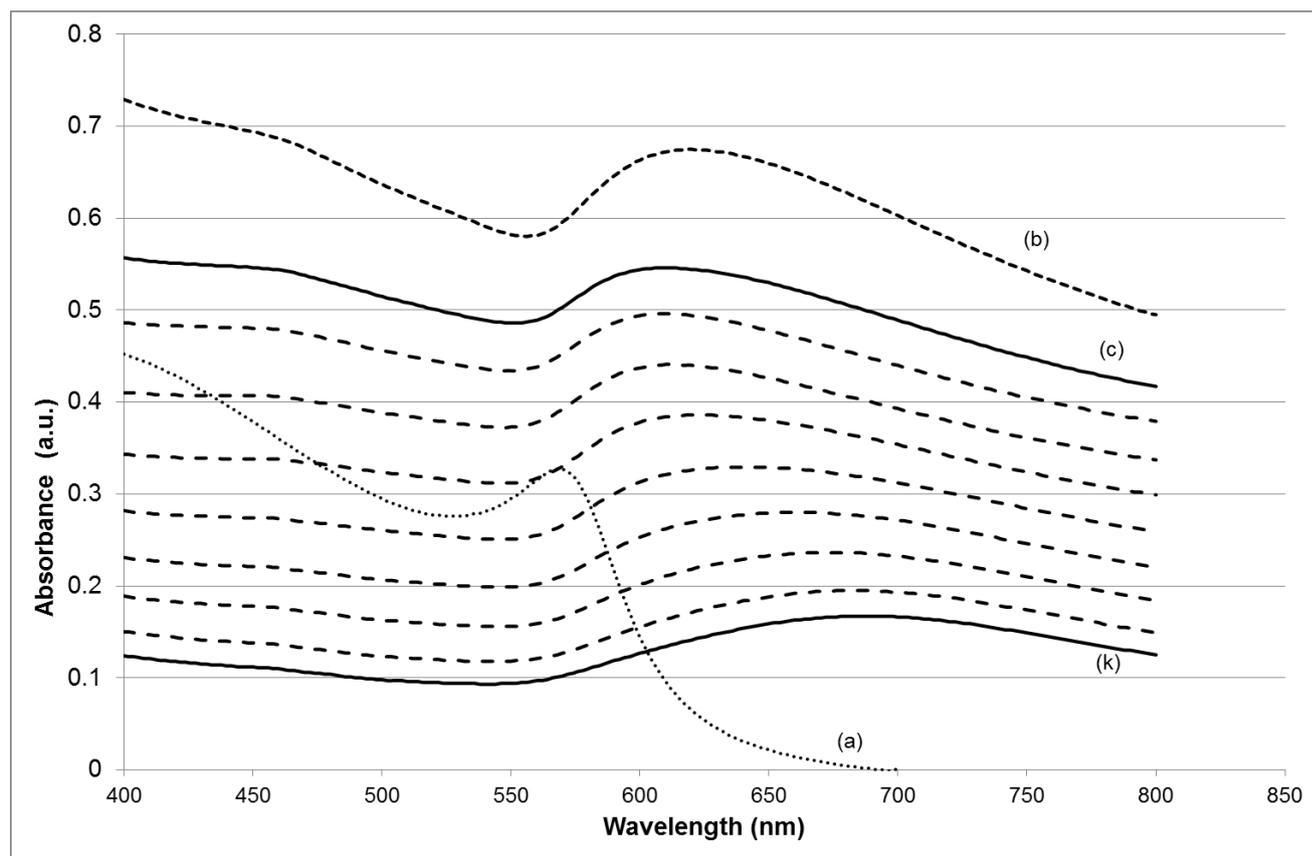
Figure 9. Absorption spectra of dispersions of Cu nanoparticles (a) chemically synthesised (0.1 ml dispersion diluted in 3 ml water), (b) copper nanopowder dispersed with 20 kHz ultrasound, (c) – (k) monitored every 3 min after the addition of glacial acetic acid. The upper and the lower solid spectra were monitored 1 min and 25 min after the addition of glacial acetic acid, respectively.
