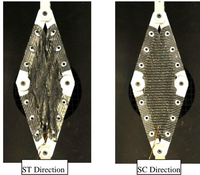
Figure 8 The images showing the influence of stitching direction during intraply shear tests of NCF reinforced prepregs determined with Picture Frame (PF) test.
