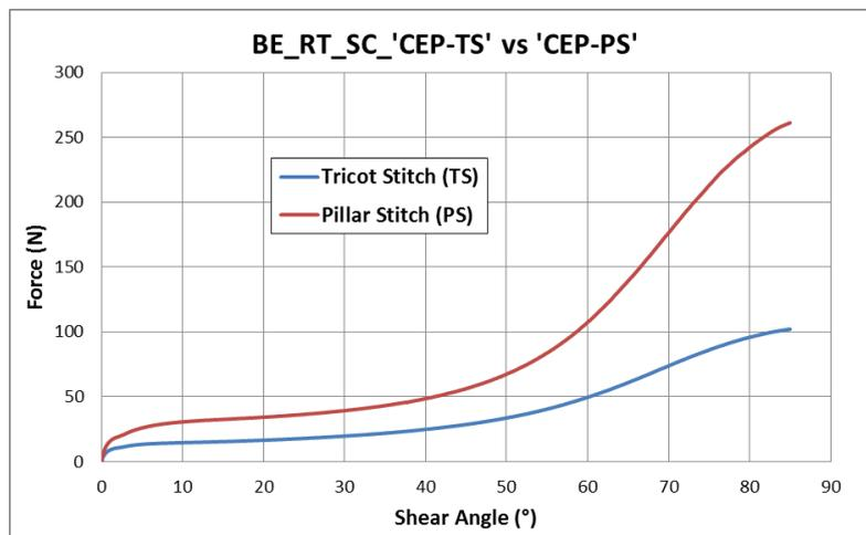
Figure 7 BE tests comparison of PS and TS Prepregs in the SC directions at room temperature (RT).
