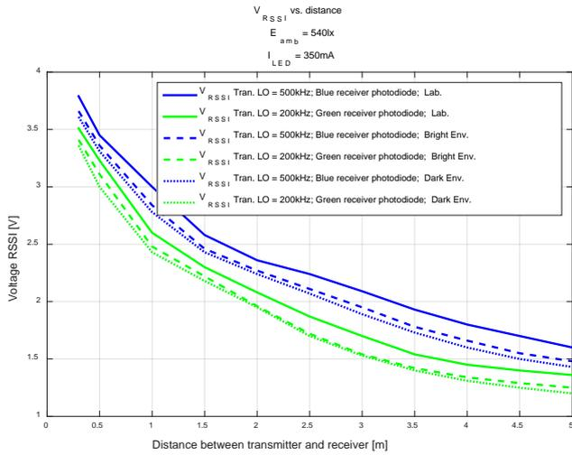
Fig. 7. Received signal strength in different distance
