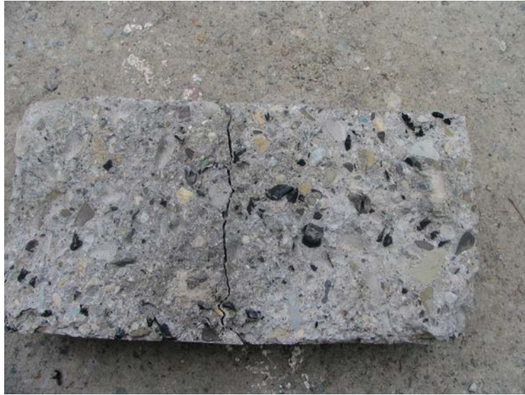
Fig. 8. Rubber particles distribution in concrete matrix after failure during tensile loading.
