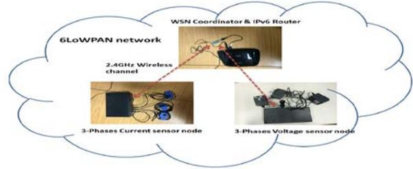
Fig.3 6LoWPAN based energy monitoring system
