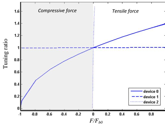
Figure 4. Comparisons of tuning ratios of scaled piezoelectric energy harvesters.
