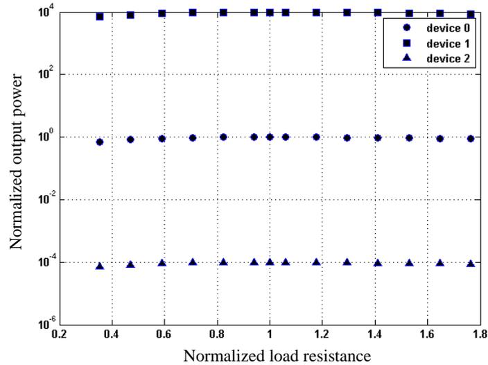
Figure 6. Comparison of output power of scaled piezoelectric energy harvesters under the constant vibration acceleration.
