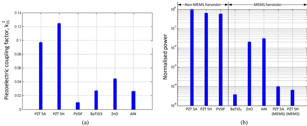
Figure 8. Comparisons of different piezoelectric materials used in energy harvesting (a) piezoelectric coupling factor (b) normalized power.
