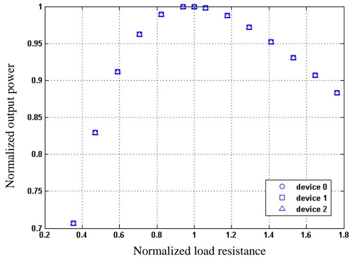
Figure 7. Comparison of output power of scaled piezoelectric energy harvesters under the constant vibration amplitude.
