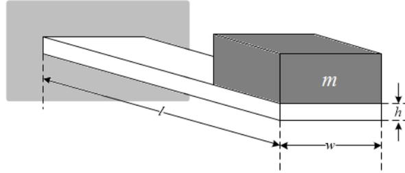
Figure 1. A cantilever beam structure.
