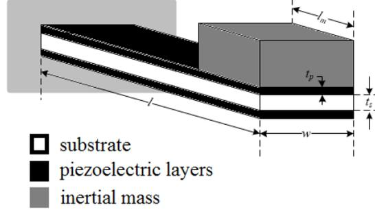
Figure 5. A cantilever based bimorph piezoelectric energy harvester.
