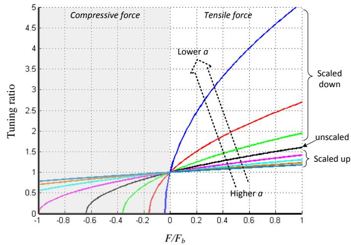
Figure 3. Tuning ratios of various scaled cantilever beams.
