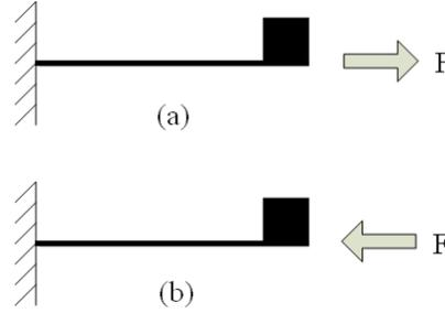
Figure 2. Resonant frequency of a cantilever structure can be tuned by applying an axial force (a) tensile (b) compressive.
