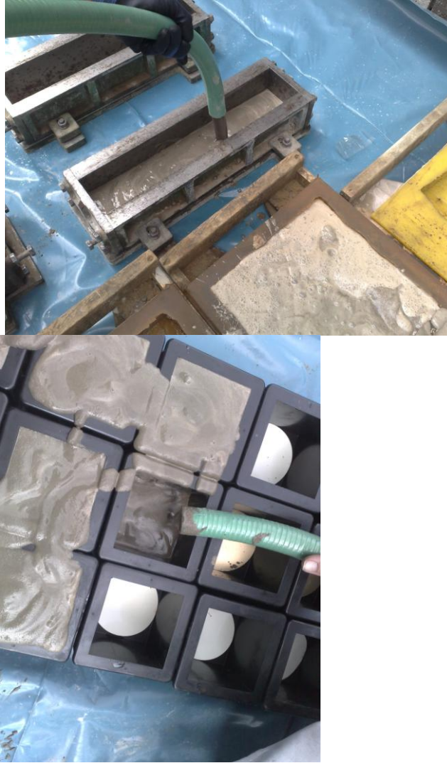
Fig.1 Aer-Tech material being poured in the moulds
