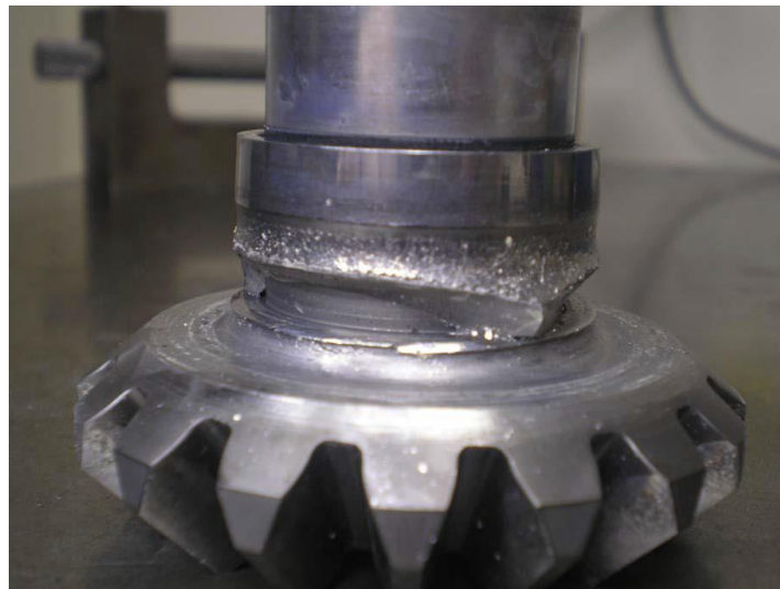
Figure 18 bearing failure progress at 24% and 30% of life time
