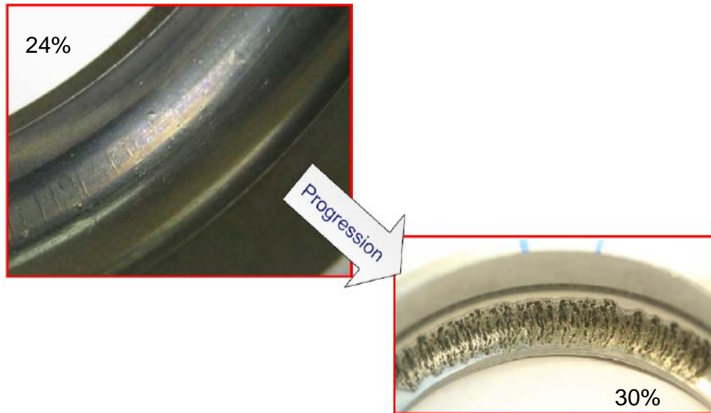
Figure 18 bearing failure progress at 24% and 30% of life time
