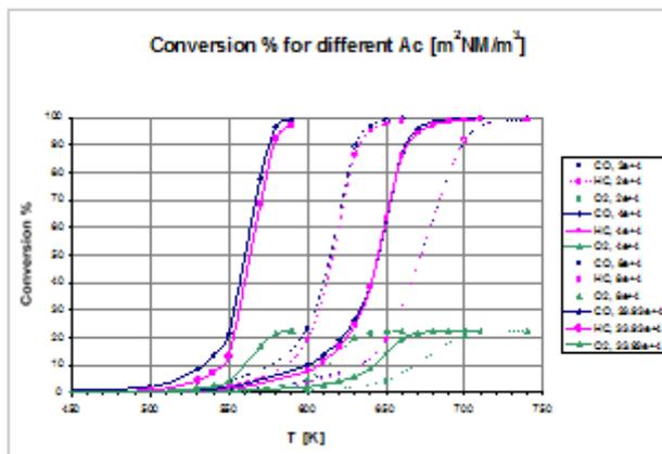
Figure 13 Single channel simulations of ageing.  $A_c$  values are shown in the key, Manolov (1999).
