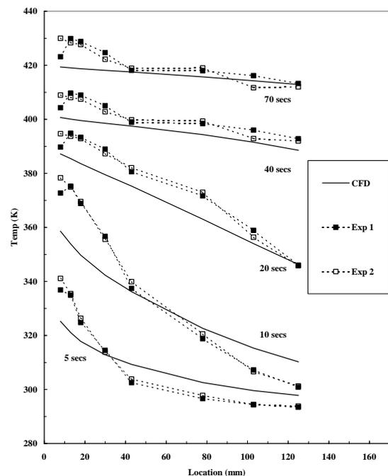
Figure 8 Measured and predicted substrate temperatures along the length of an axi-symmetric converter during warm up, Benjamin and Roberts (1999).
