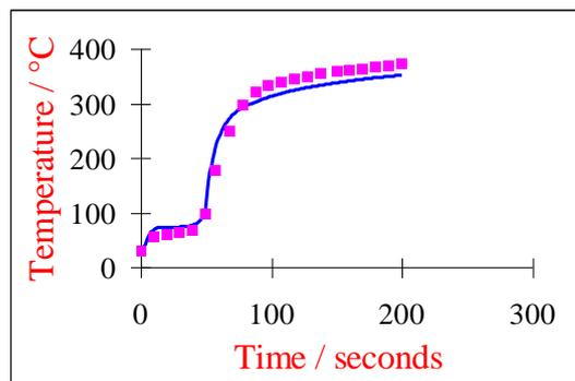
Figure 12 Predicted and measured temperatures in a converter during light-off. Clarkson and Benjamin (1995)
