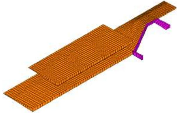
Figure 7 Typical computational mesh for simulating catalyst warm-up.
