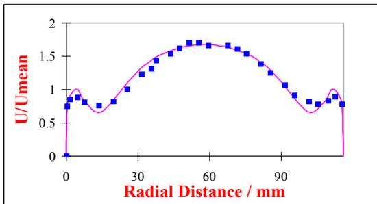
Figure 6 Measured and predicted velocity profiles at the exit of an axi-symmetric converter.
