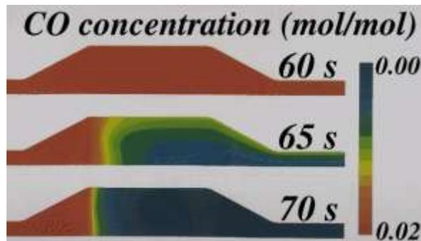
Figure 11 Predicted concentration of CO during light-off.
