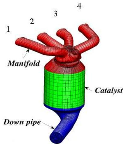
Figure 3 Typical configuration of a close-coupled catalyst.
