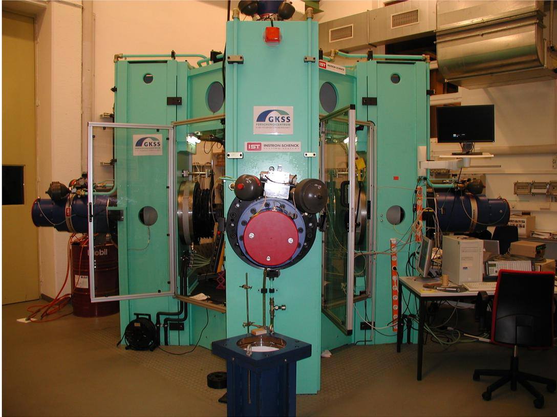
(a) Instron triaxial testing machine used in this study
