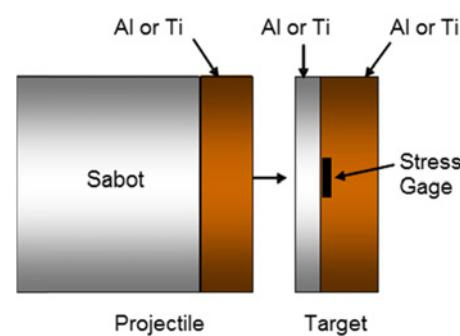
**Fig. 4** Schematic of flyer plate test setup
