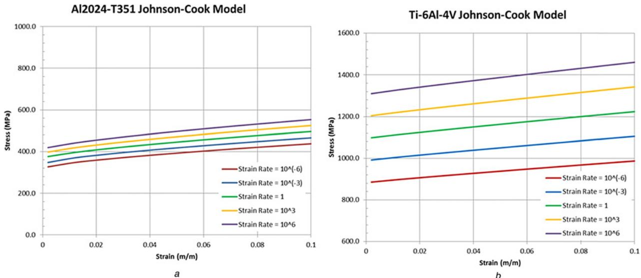
**Fig. 2** Johnson-Cook plots of yield stress as a function of strain rate for Al2024-T351 and Ti-6Al-4V
