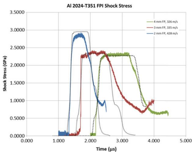
**Fig. 8** Comparison of the predicted and measured flyer plate impact shock response (AI 2024-T351)
