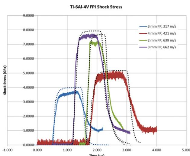
**Fig. 9** Comparison of the predicted and measured flyer plate impact shock response (Ti-6Al-4V)
