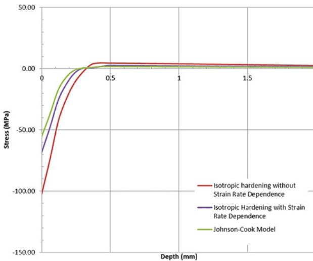
**Fig. 1** Effects of strain rate on predicted residual stress profiles from LP simulation
