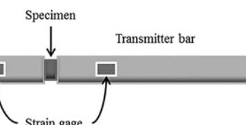
bar. For a striker bar of length  $l_s$ , the pulse duration is given by
