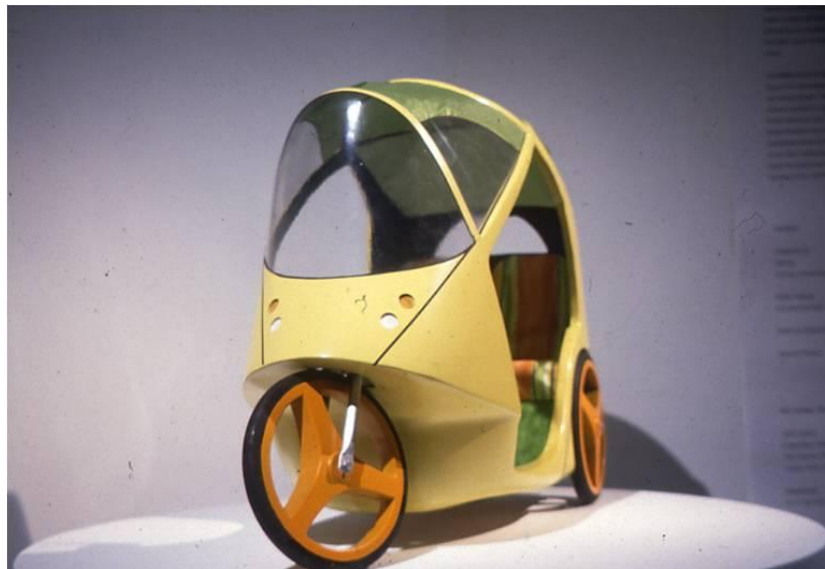
The earliest physical model (1/4 scale) on show at the Oxo Tower, South Bank, London. It was intended to be a pedal/electric hybrid.
