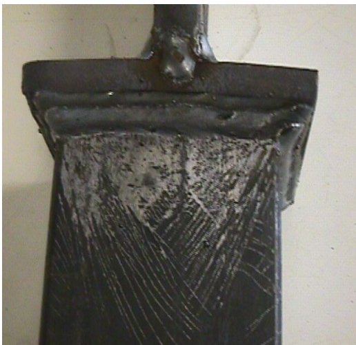
Fig. 6 Typical tube yielding (Test 3, see Table 2)
