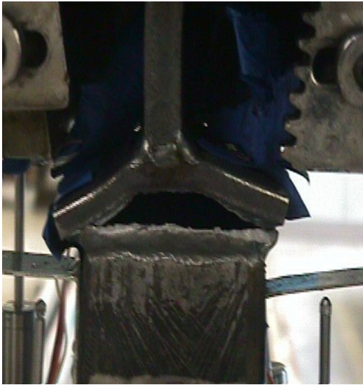
Fig. 5 Cap plate-to-tube weld fracture (Test 1, see Table 2)
