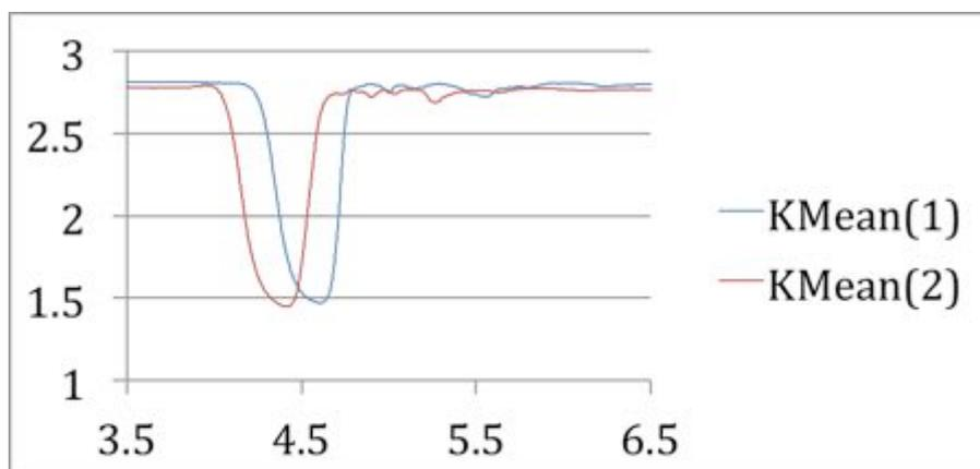
Figure 2. Permittivity against time in seconds for two planes of ECT separated by 6 cm.
