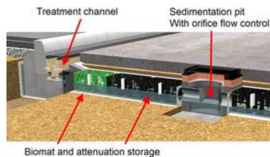
Figure 2: Schematic Section Through Channel based MPPS
