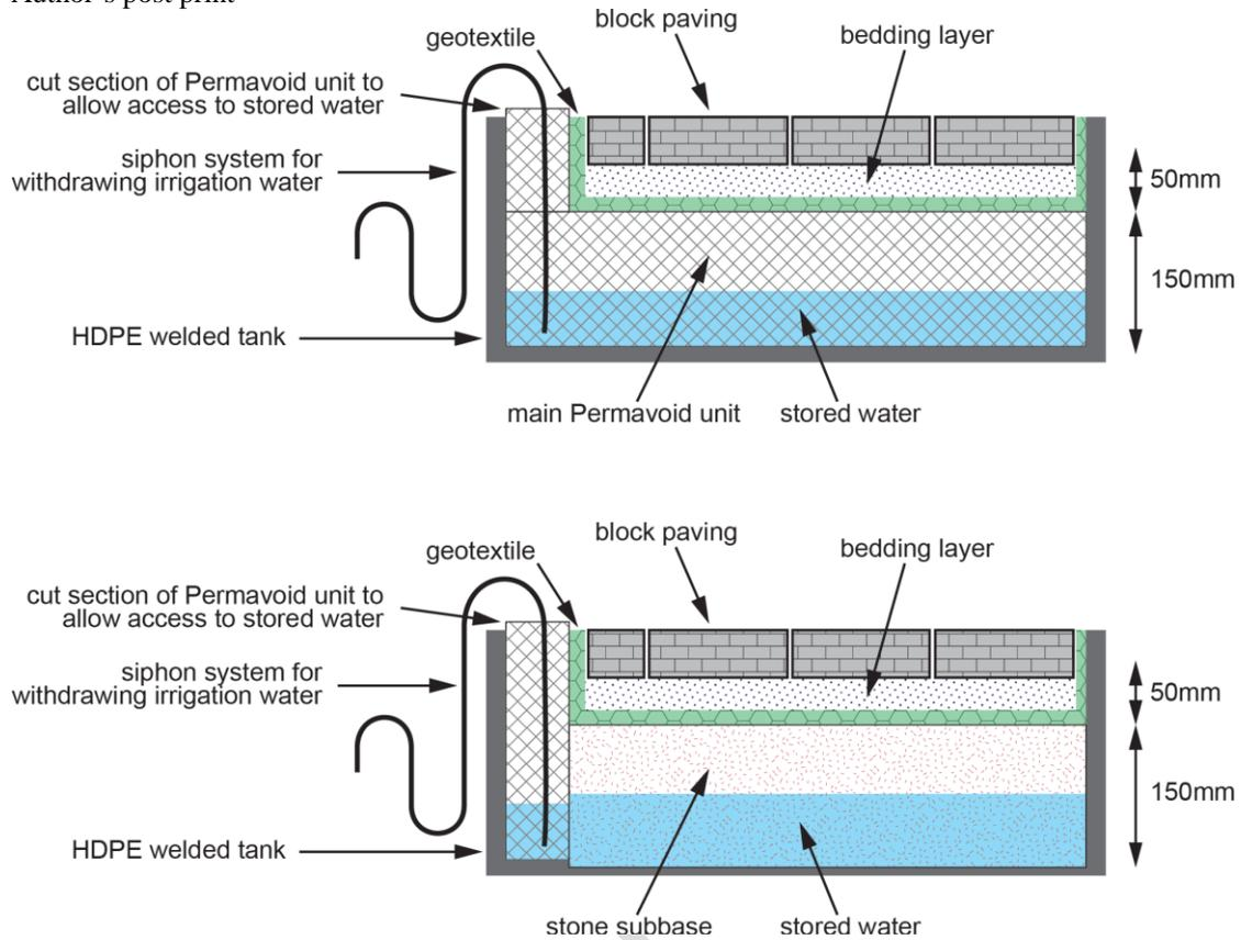
Figure 1 Schematics of the Rig Model Types: Top-Permavoid Bottom–Stone Sub-base
