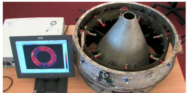
Figure 5: Base station and instrumented gas turbine engine
