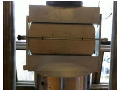
Fig. 7: Splitting test on cylindrical specimen
