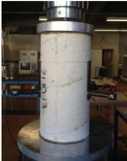
Fig. 4: Compression test on a (16D x 32H) specimen
