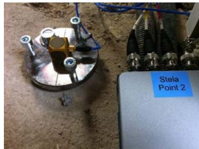
Fig. 9 : Vibrational measurements by triaxial accelerometers.
