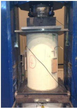
Fig. 6: Compression test on a (30 cm-D x 55 cm-H) specimen
