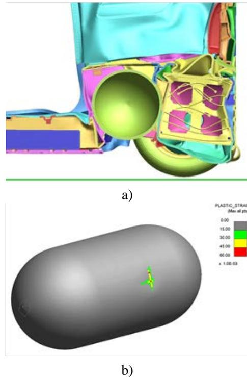
Figure 11 a) Microcab rear structure rotation, b) Contact with fuel tank.
