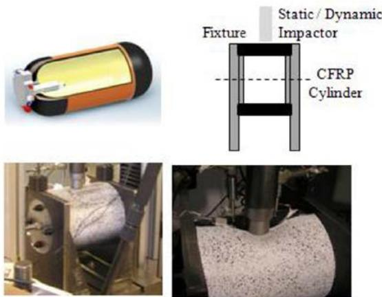
Figure 4 Level 3 CFRP cylindrical test setup [3]
