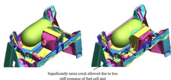
Figure 12 Fuel cell orientation
