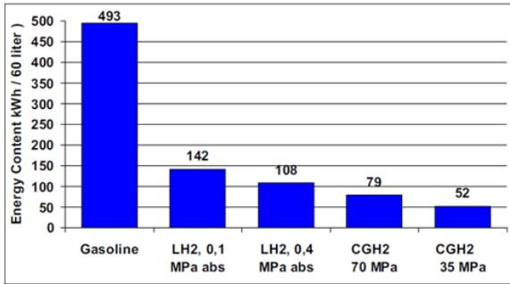
Figure 3 Energy content in 60 litre tank [1]
