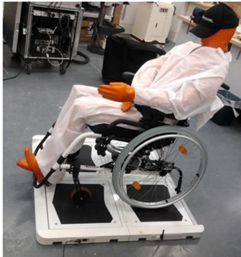
Fig. 4. The WheelSense measurement platform
