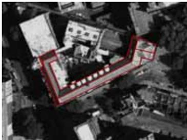
Figure 4: roof edge detection final results using method/algorithms
