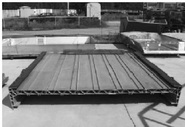
**Fig. 1** A section of extruded aluminium train floor structure (Fig. 8 in Ref. [14])
