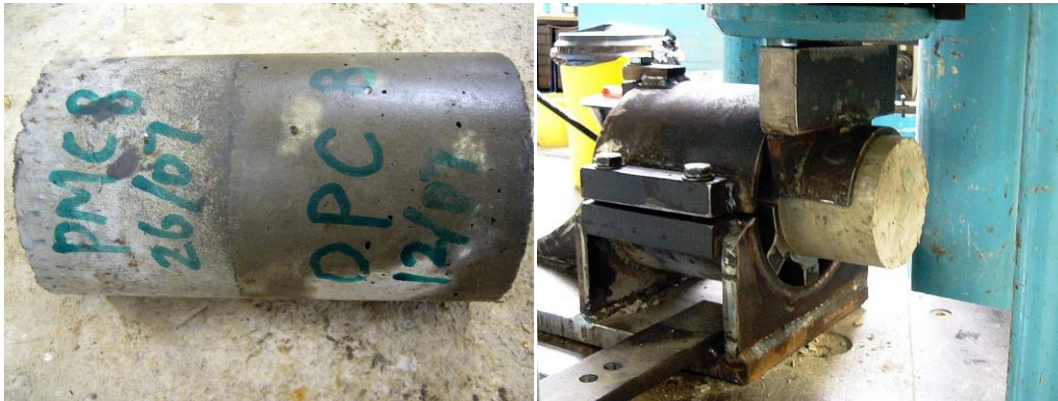
Figure 3.3 Cylinder Direct Shear Test (a) Sample (b) Testing Rig
