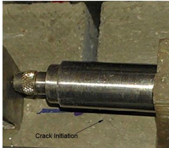
Figure 4.27 Crack Initiaton in PVAPMC Beam 1
