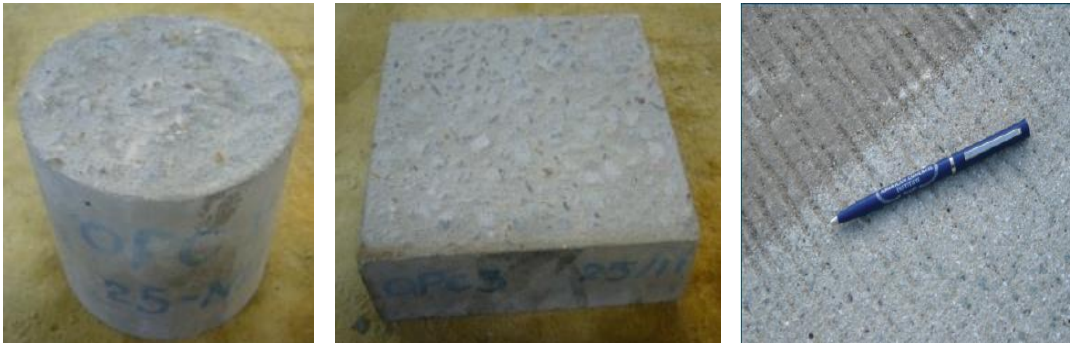
Figure 3.15 Surface Texture of OPCC in Lab(a) & (b) and in Real Site (c) 6
