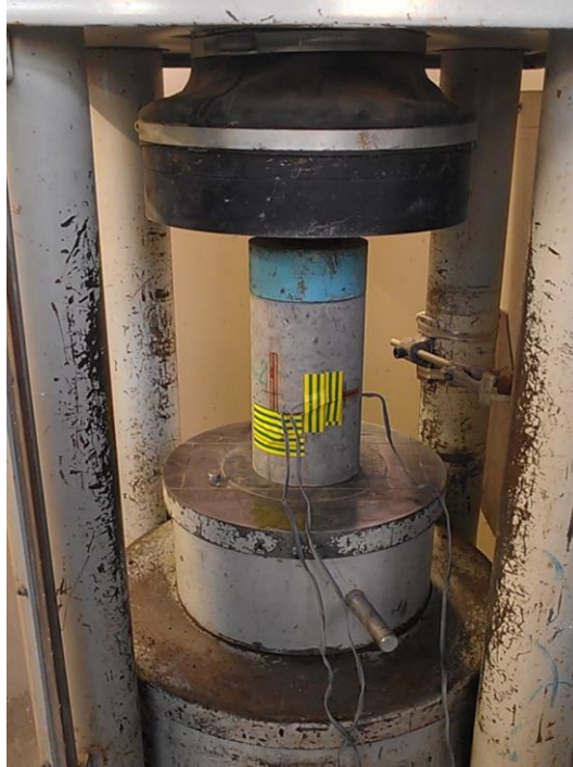
Figure 3.18 Test for E-value and Poisson's Ratio
