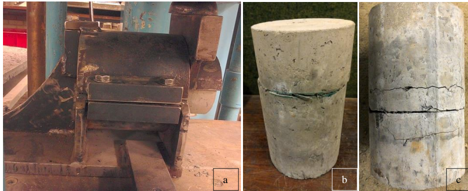
Figure 4.9 (a) Cylinder Direct Test (b) Failure Plane (c) Lift Joint Cracking
