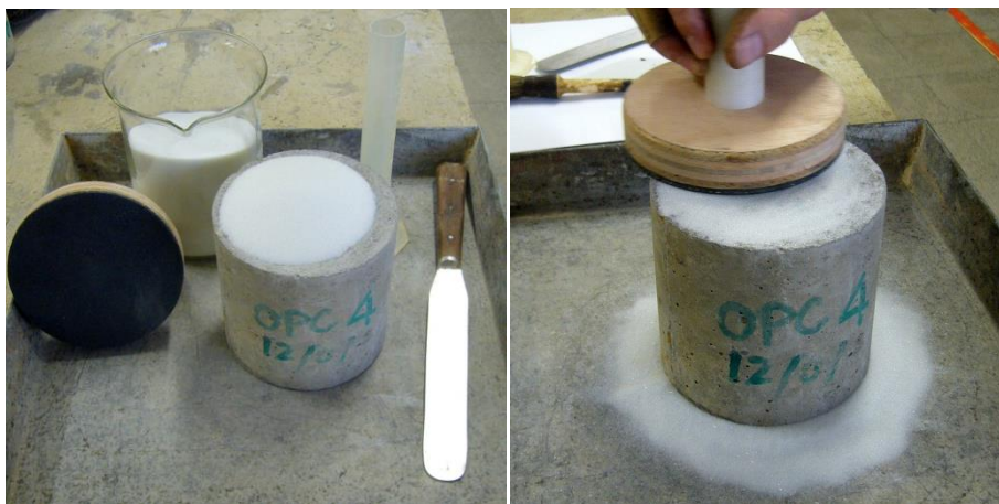
Figure 3.16 Sand Patch Method (a) Apparatus (b) Test in Progress
