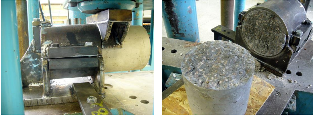
Figure 4.6 Cylinder Direct Shear Test (left); Failed Section (PMC2 p ) (right)
