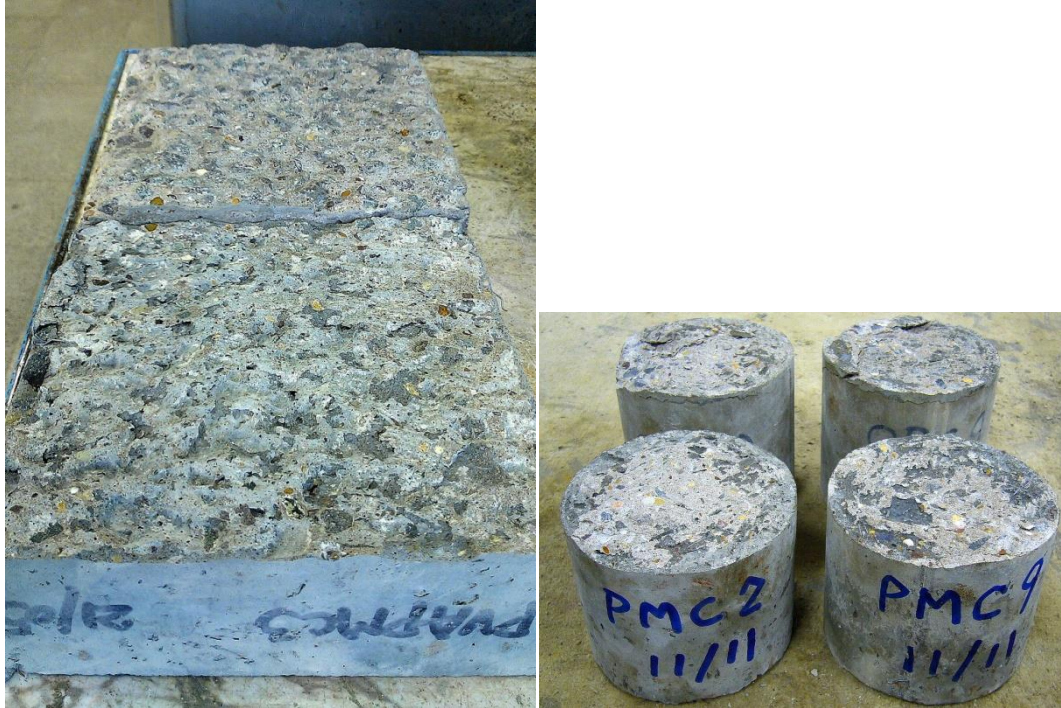
Figure 3.11 Failed Interfaces: (a) Block Splitting Test. (b) Cylinder Shear Test
