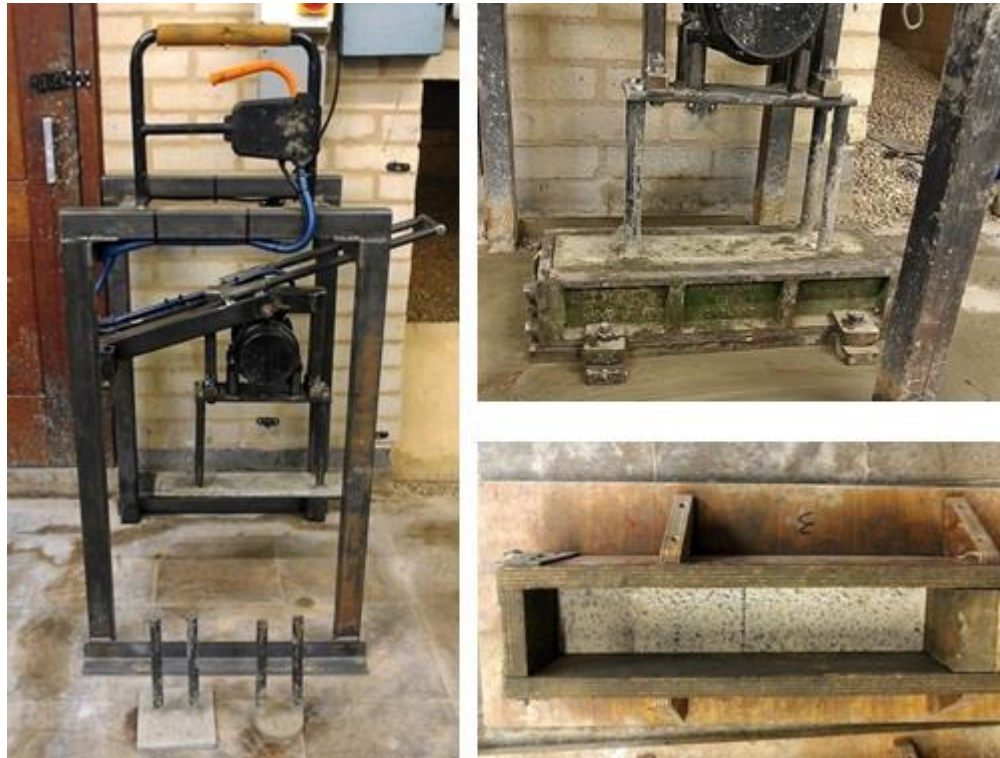
Figure 3.14(a) Vibrating Compactor and Attachments (left) (b) Beam Compaction (top right) (c) Composite Beam Moulds (bottom right)
