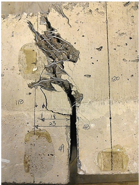
Figure 4.32 Failure Cracks in SBRPMC Compo. Beam 2
