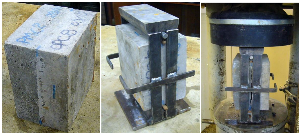
Figure 3.2 Block Splitting Test (a) Sample (b) Jig (c) Subject to Splitting
