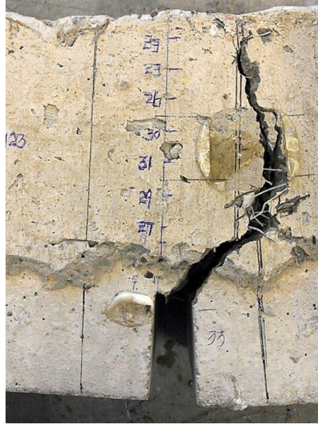
Figure 4.38 Failure Cracks in PVAPMC Compo. 30 Beam 1
