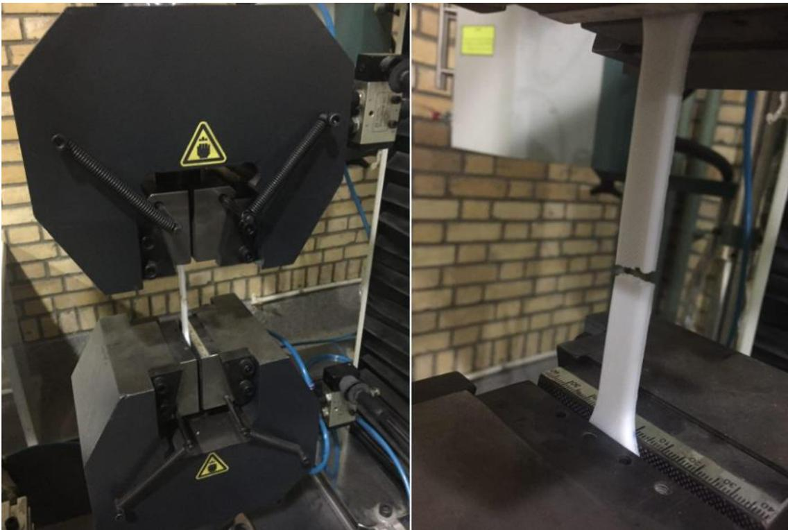
Fig. 4. Brittle fracture of the specimen (sample #12)
