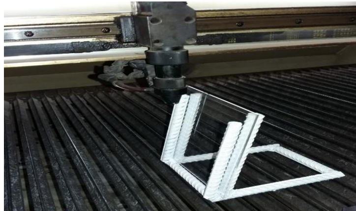
Figure. 4. Experimental determining the focal plane position of the used CO 2 laser machine
