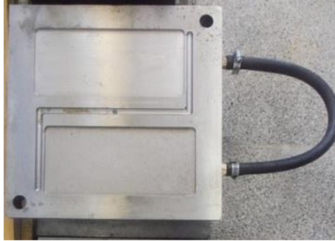
Figure. 3. Used mold for injecting the polycarbonate specimens
