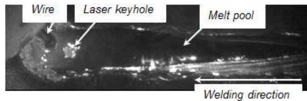
Fig. 3: Typical high speed image of the LHAW process (the wire diameter is 1.2mm)
