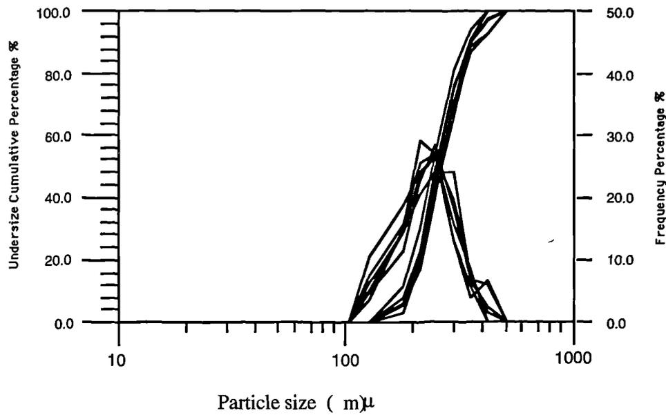
Figure 2.5 4 measurements of sand B with the Optomax
