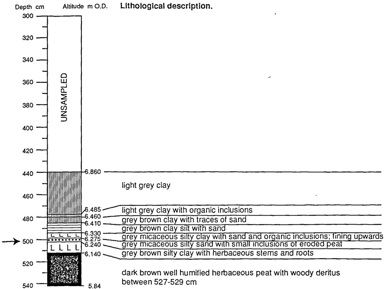
Figure 5.80. Lithostratigraphy of core 5B at Moniack. The arrows mark the core section analysed.
