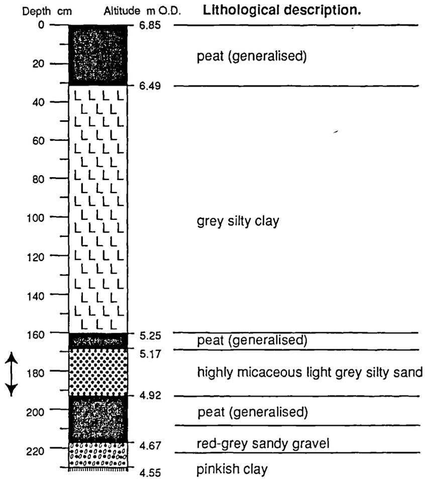
Figure 5.72. Lithostratigraphy of core 3 at Fullerton. The arrows mark the core section analysed.
