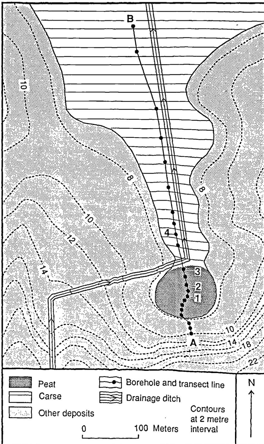
Figure 5.64. Borehole Locations at the Fullerton Gully
