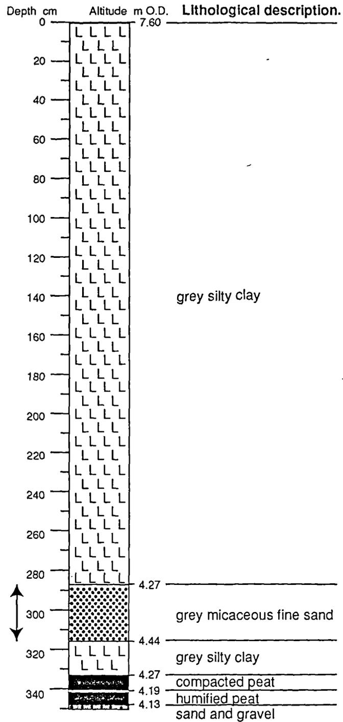
Figure 5.74. Lithostratigraphy of core 4 at Fullerton. The arrows mark the core section analysed.
