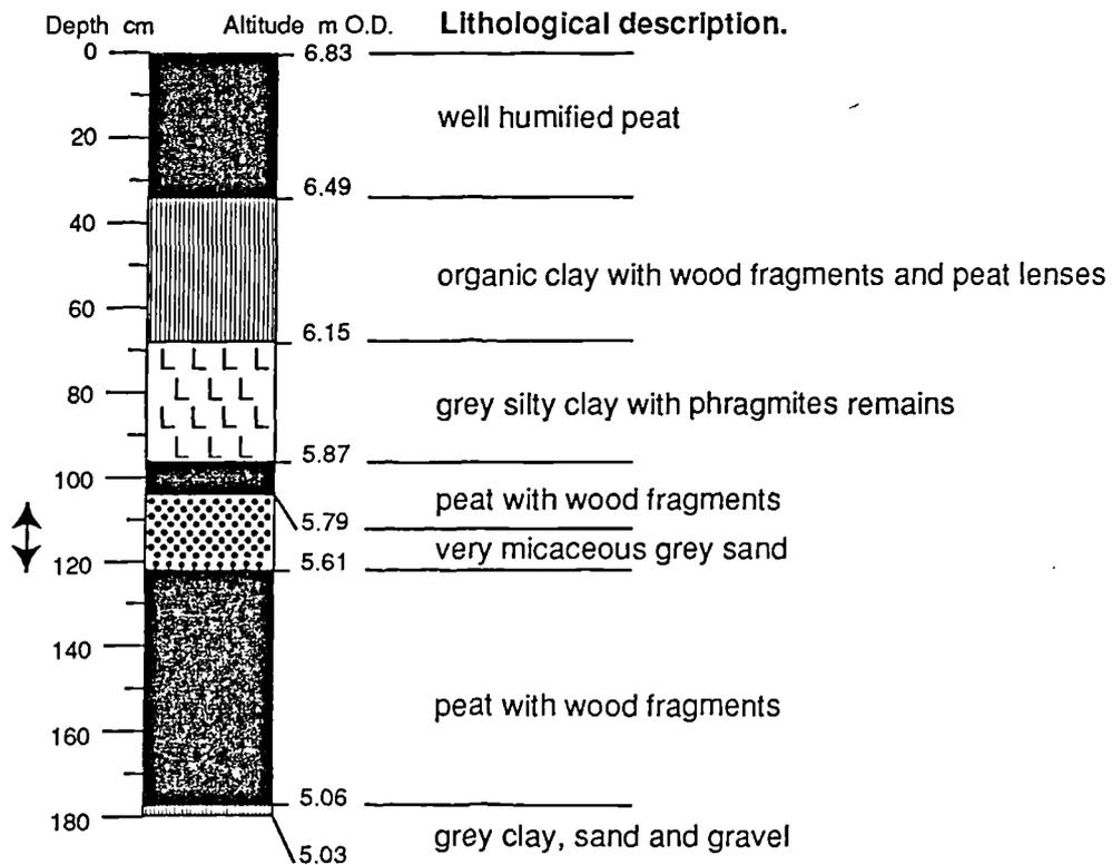
Figure 5.68. Lithostratigraphy of core 1 at Fullerton. The arrows mark the core section analysed.
