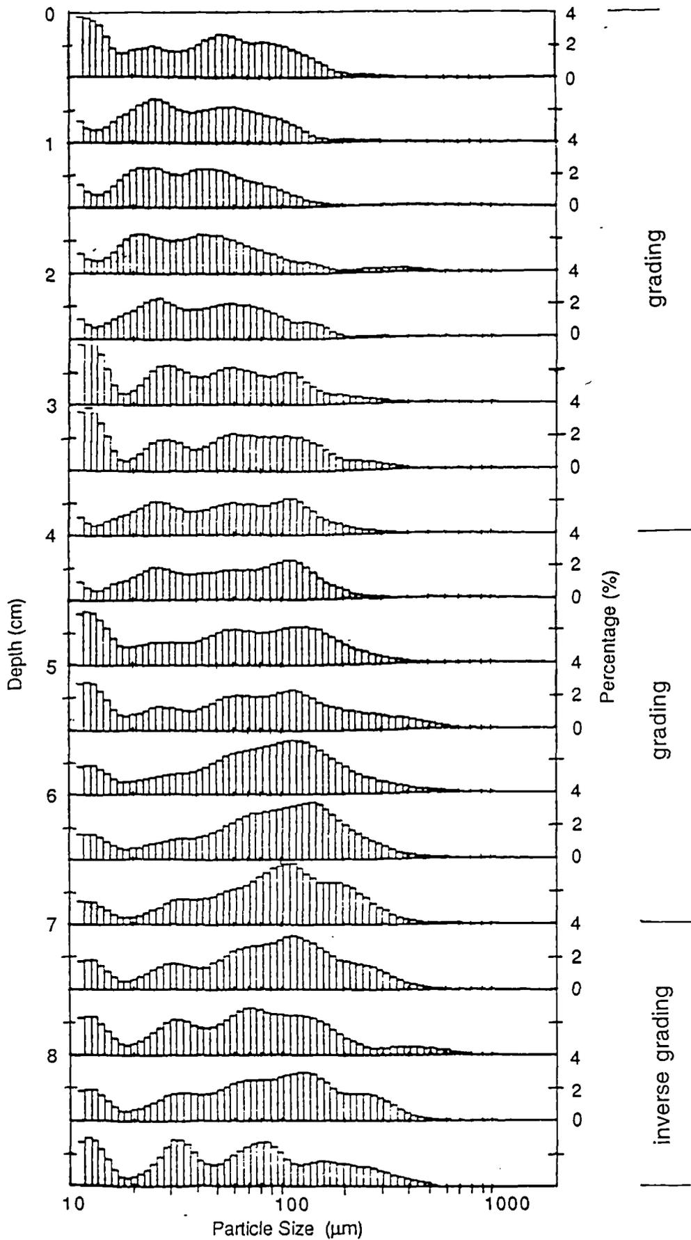
Figure 5.81. Upcore progression of particle size histograms within the sand layer at Borehole 5B, Moniack (Figure 5.80).
