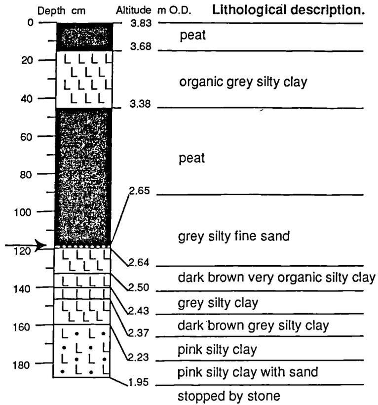
Figure 5.86. Lithostratigraphy of core 63 at Tarty Burn. The arrow marks the core section analysed.
