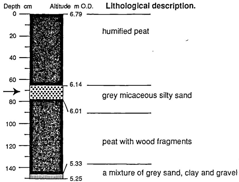
Figure 5.70. Lithostratigraphy of core 2 at Fullerton. The arrow marks the core section analysed.
