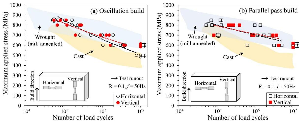
Fig. 4. Maximum applied stress vs load cycles (S-N curves) for oscillation and parallel pass build strategies. Encircled data points indicate crack initiation from a surface pore. Best fitted lines are drawn. Conventional manufactured Ti64 wrought [20] and cast [20] are also shown.
