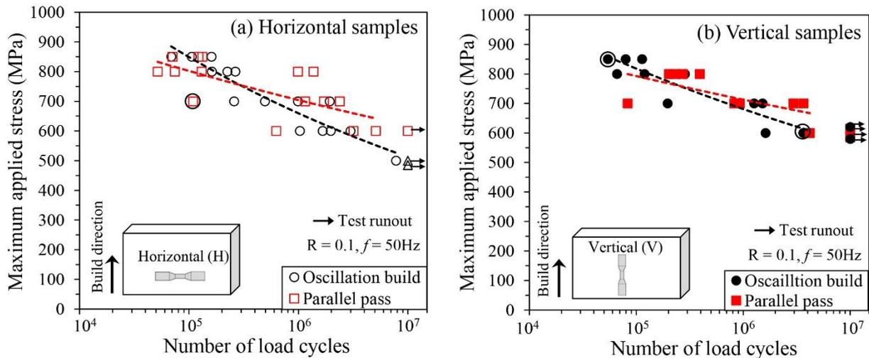
Fig. 5. A comparison of S-N data along with the best fit curves (dashed lines) for both build methods in horizontal and vertical orientation. Encircled data points indicate crack initiation from a surface pore
