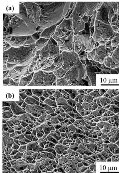
Fig. 11. Fracture surfaces of tensile test samples: (a) oscillation (b) parallel pass builds
