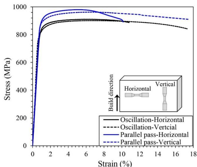
Fig. 3. Average tensile test curves for oscillation and parallel pass build samples.
