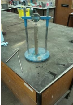
Figure 4.45: Dial gauge measuring mortar bar Figure 4.46: Specimens sulphate attack
