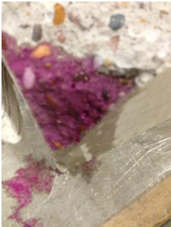
Fig 5.43 Binder Mix Concrete Sample (0.5 W/B) Dry Cured - 3mm Carbonation
