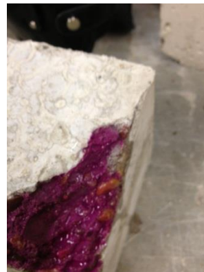
Fig 5.38 Pure OPC Mix Concrete Sample (0.5 W/B) Dry Cured - 0.5 mm Carbonation
