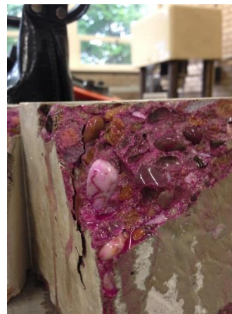
Fig 5.38 Pure OPC Mix Concrete Sample (0.5 W/B) Dry Cured - 0.5 mm Carbonation
