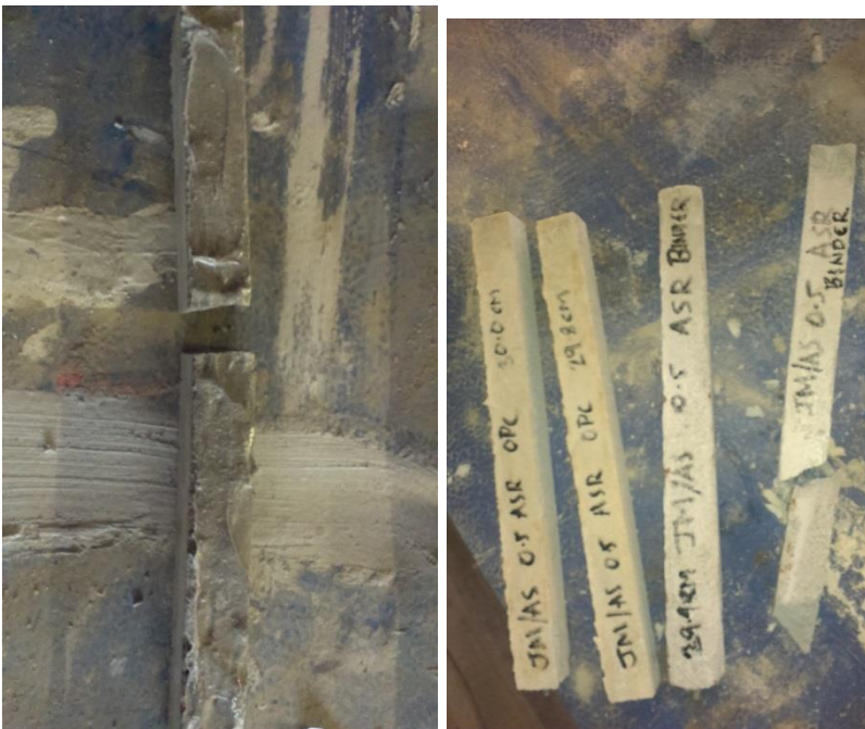
Figure 5.59: failure of mortar bar
