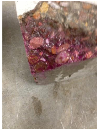
Fig 5.444 Pure OPC Mix Concrete Sample (0.6 W/B) Wet Cured – 0.5mm Carbonation
