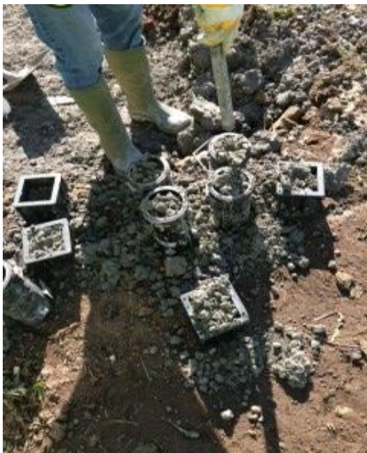
Figures 4.37: Compaction and Sample Taking
