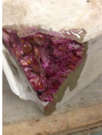
Fig 5.42 Pure OPC Mix Concrete Sample (0.5 W/B) Dry Cured – 0.5mm Carbonation
