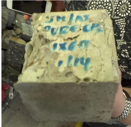
Figure 5.23: compressive strength failure pure OPC
