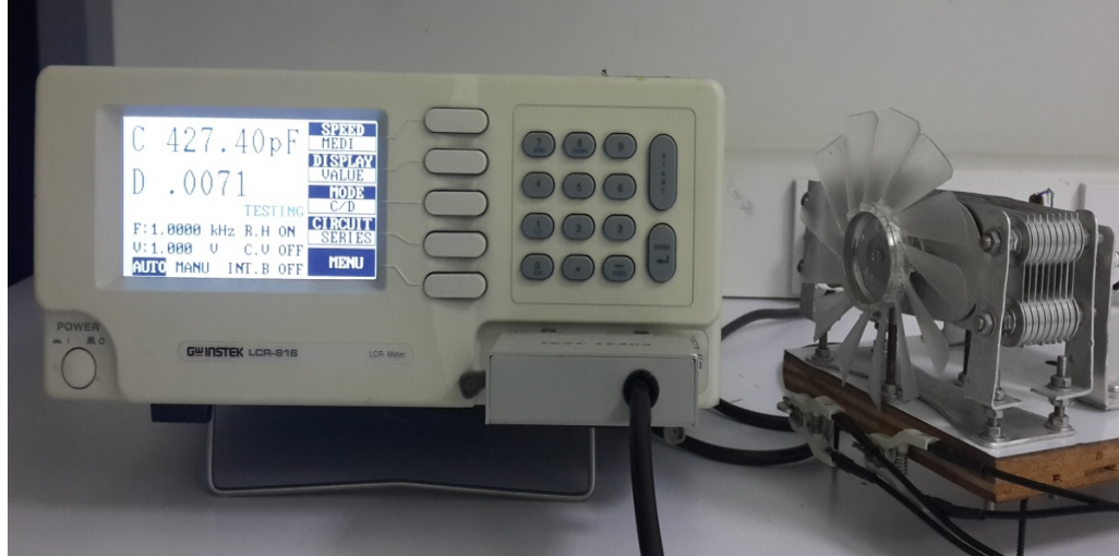
Figure 6.36: LCR meter and the variable capacitor prototype
