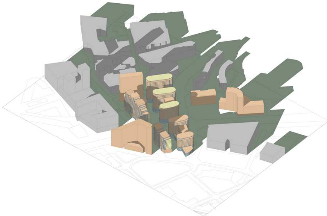
Figure 13 – IES model of Masshouse for measuring direct sun access through Winter Possible Sunlight Hours
