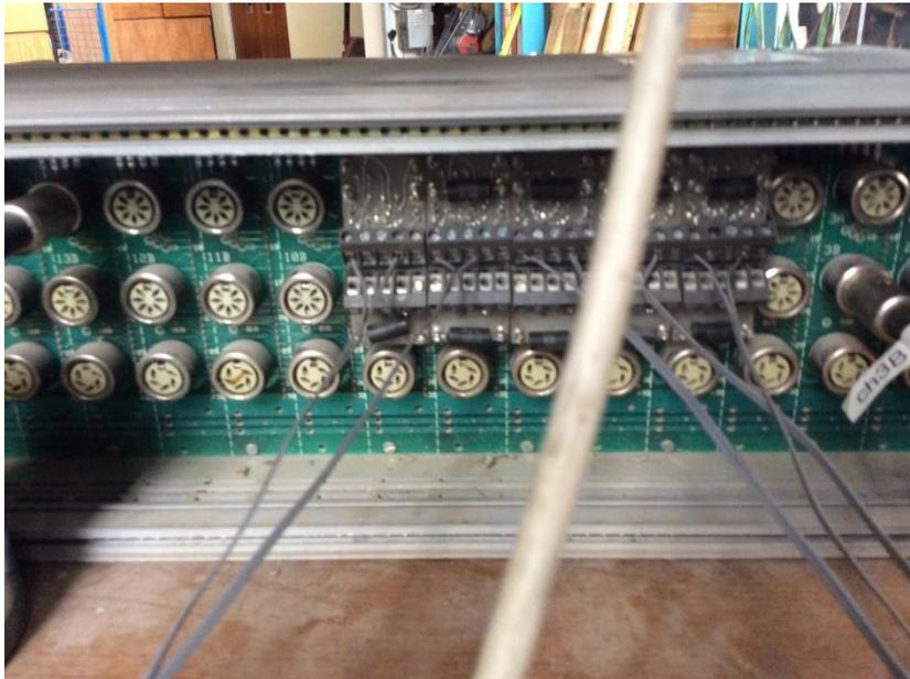
Fig 7.8: ERGs strain gauges connection to data logger.
