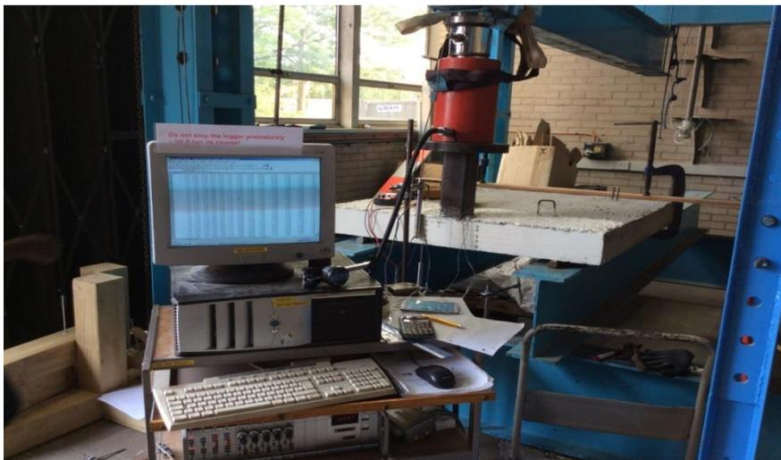
Fig 7.1: Photo of Test set up for slab 1. .
