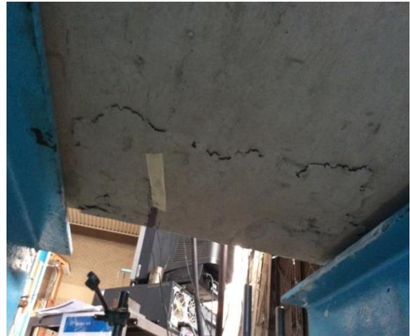
Fig 7.9 a: Punching shear of the connection Fig 7.9b: crack periphery (bottom)
