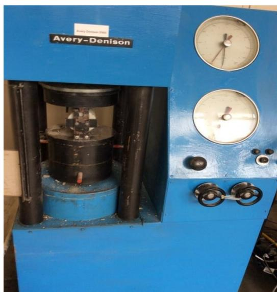
Fig 7.4: Splitting tensile test
