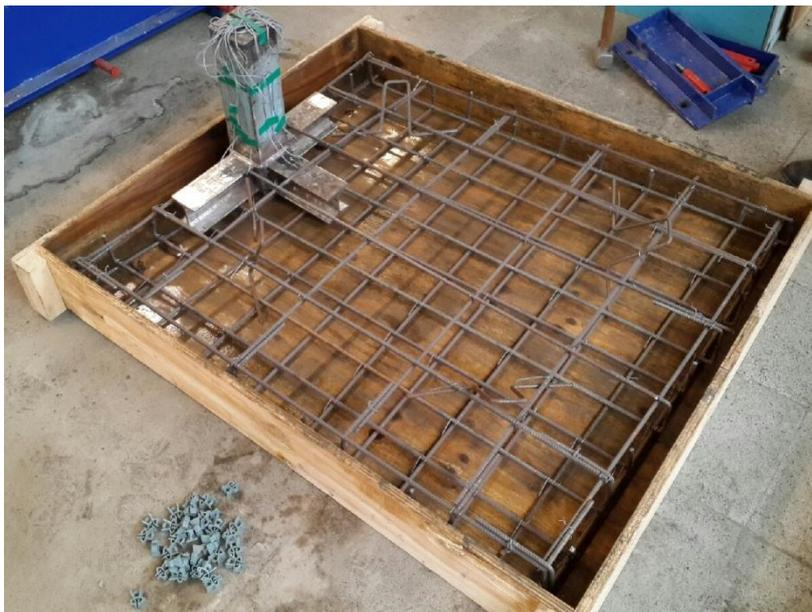
Fig 7.18: photo of shearhead inserted between reinforcement grids
