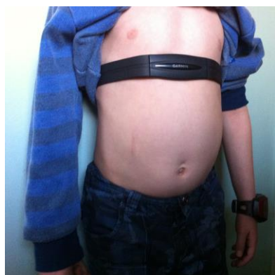
Figure 5.1 Monitor placements for integrated GPS and HR monitor
