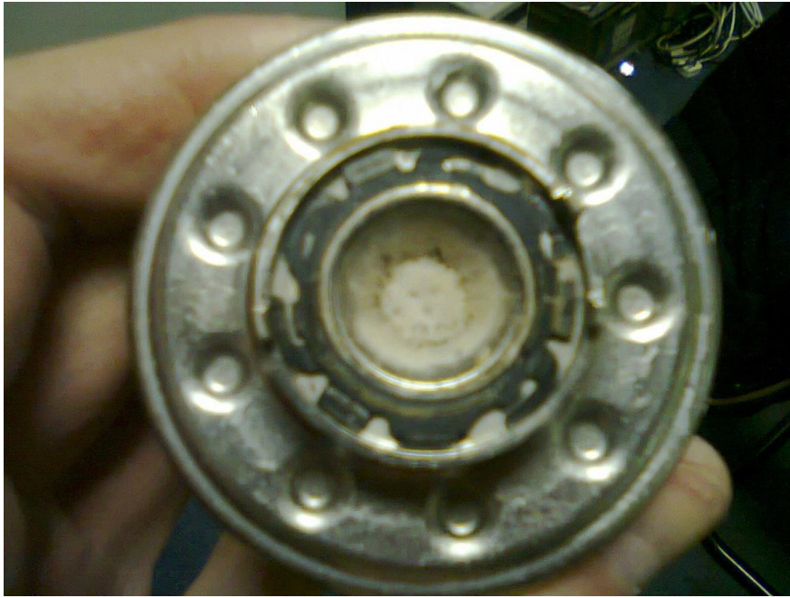
Figure A.6 Deposit on the tip of the injector after ~200 minutes spraying.
