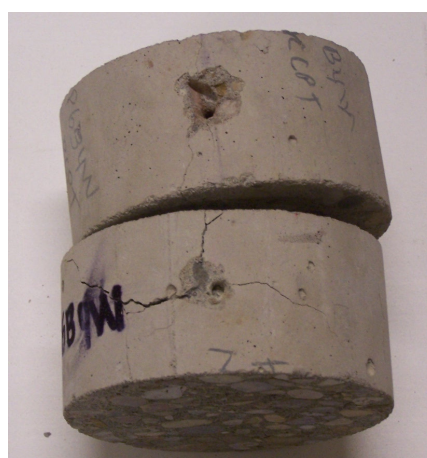
Figure 11-18 BPD sample cracked during drilling
