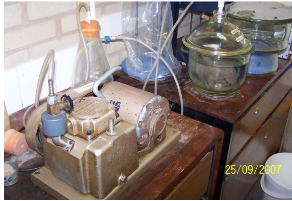
Figure 6-17 Vacuum pump and desiccator used to saturate concrete specimens
