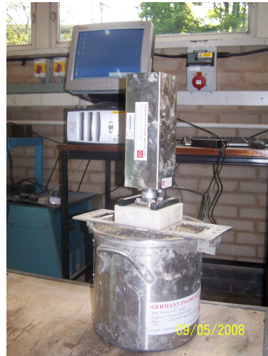
Figure 10-2 ICAR rheometer used in this research
