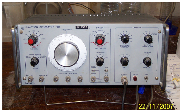
Figure 6-20 A.C. Signal generator used to measure resistivity
