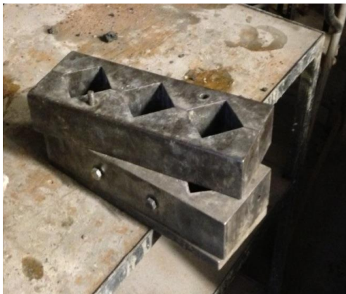
Figure 3.13 50mm moulds construction (Showing a gang of 3 moulds)
