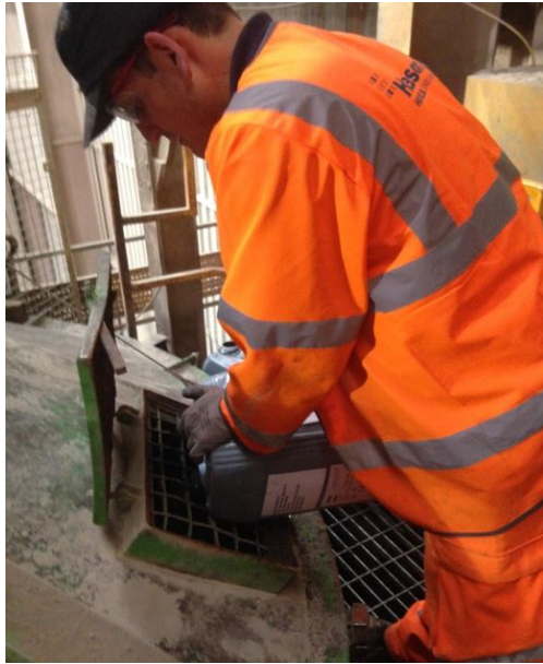
Figure 7.1 Introduction of slurry SF to the mix
