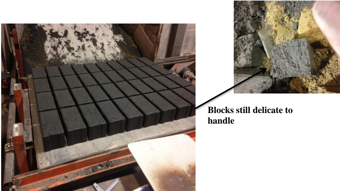
Figure 7.5 Blocks are measured to ensure the height is between 80\pm 2\text{mm}
