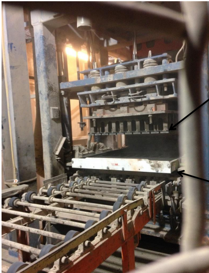
Figure 7.3 Material laid into moulds ready to be compressed and vibrated simultaneously.
