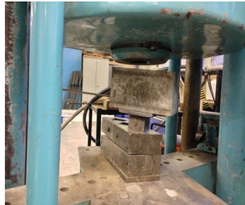
Figure 3.14 50mm cube compaction at 52KN, each were loaded and compacted individually.
