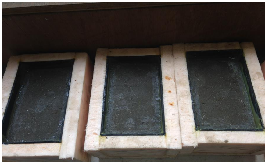
Figure 6.4 blocks after 28 freeze cycles for mix containing PC60/GGBS25/SF15
