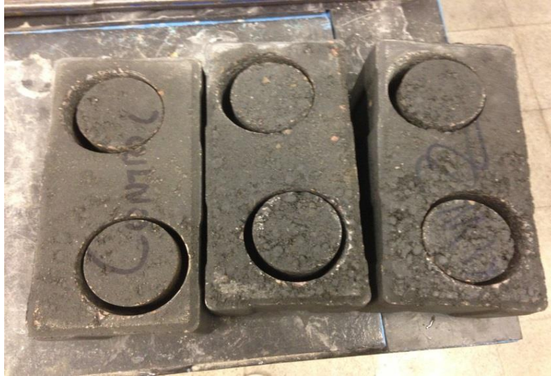
Figure 3.21 50mm cores drilled from blocks
