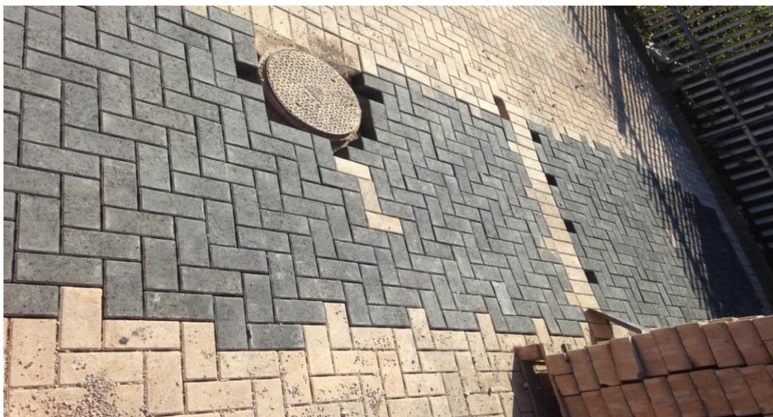
Figure 7.10 Mix 1 and 2 laid on test bed
