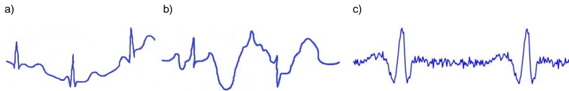
Figure 5.7 Examples of noise contaminated ECG: a) baseline drifts changes, b) motion artefacts, c) muscular/skeletal noise
