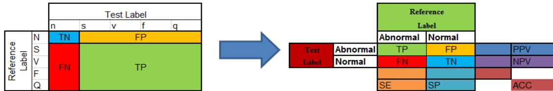
Figure 8.5 Multiclass confusion matrix to binary confusion matrix decomposition.
