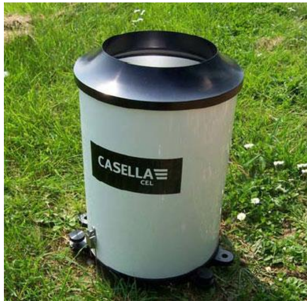
Figure 3-15 Casella tipping bucket rain gauge installed at Hope Hamilton School, Leicester.
