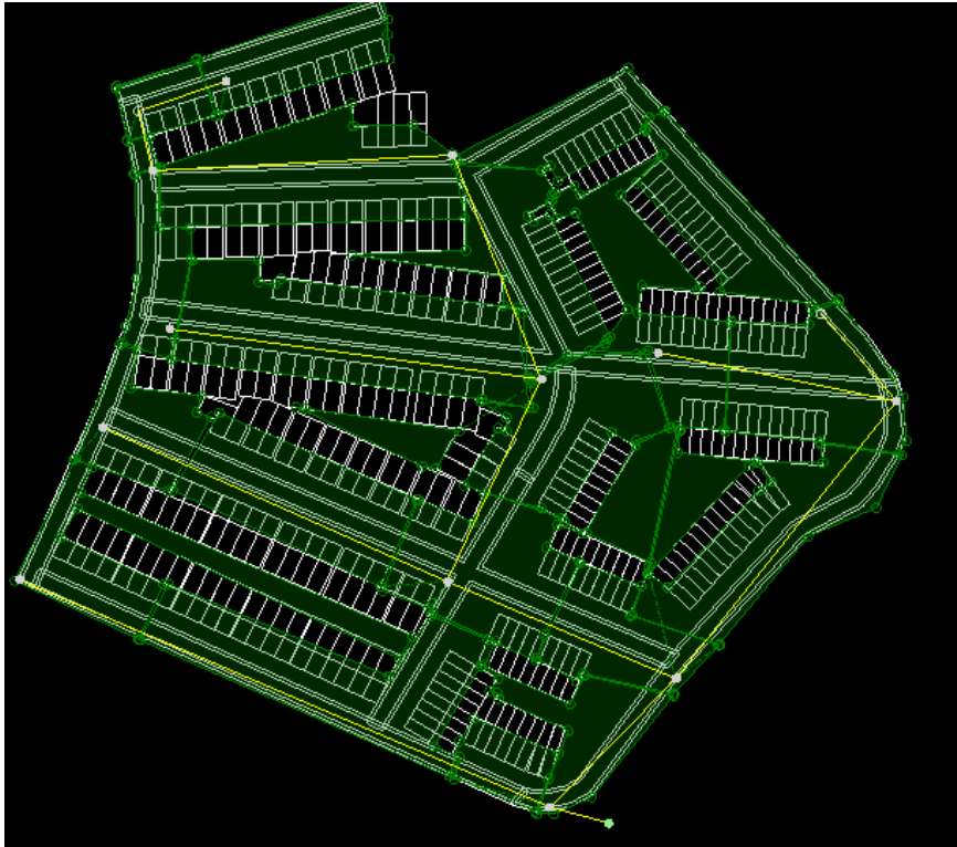
Figure 3-6 Pipe layout created in MicroDrainage at Prior Deram Park, Coventry. Yellow lines are the pipes, the green areas are the contributing runoff areas.
