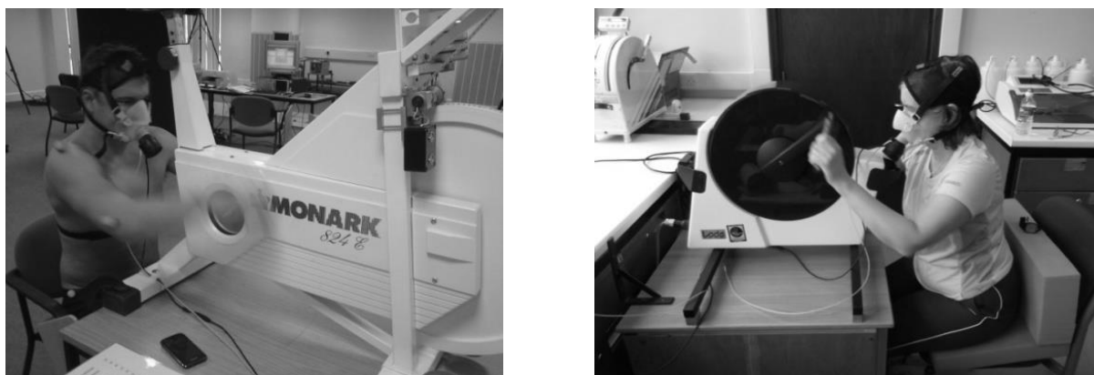
Figure 3.1: The upper body exercise set up for the modified cycle ergometer (left) used in study 1 and electronically braked arm crank ergometer (right) used in studies 2 & 4
