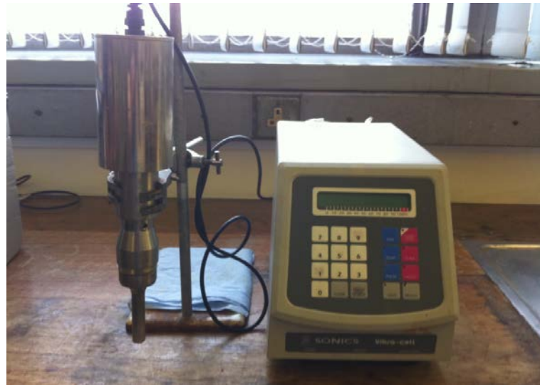
Figure 6.2b 20 kHz VCX 600 Probe set up diagram
