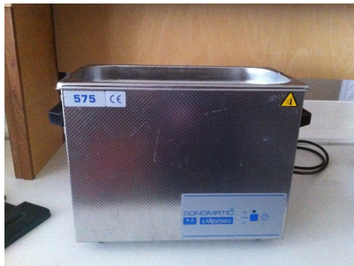
Figure 6.3a 40 kHz 475TT bath (Langford ultrasonics)
