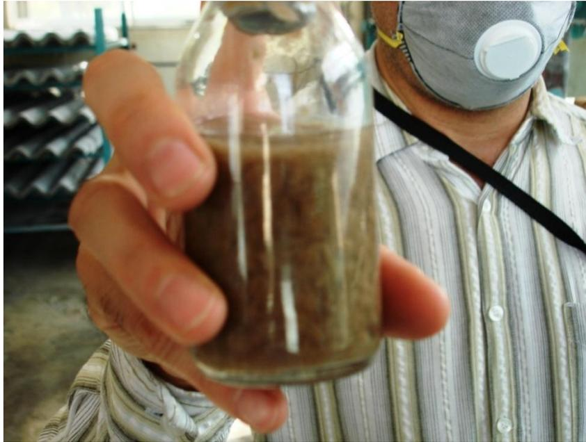
Figure 6-3 Visual inspection of pulp quality to make it usable in Hatschek machine
