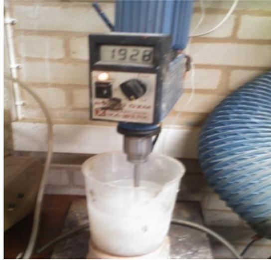
Figure 4-9 Overhead propelling mixer to unravel the natural fibres
