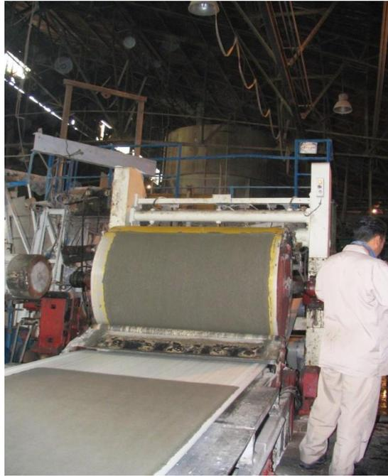
Figure 4-3 Photograph of the function of the accumulator roll in making a cement sheet with the desired thickness
