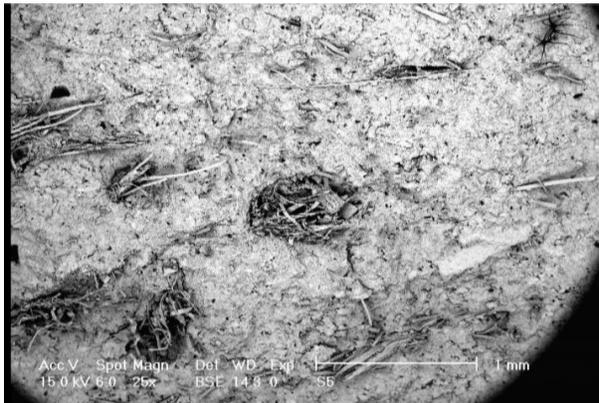
Figure 5-41 Balling (clumping) of fibres in cement matrix
