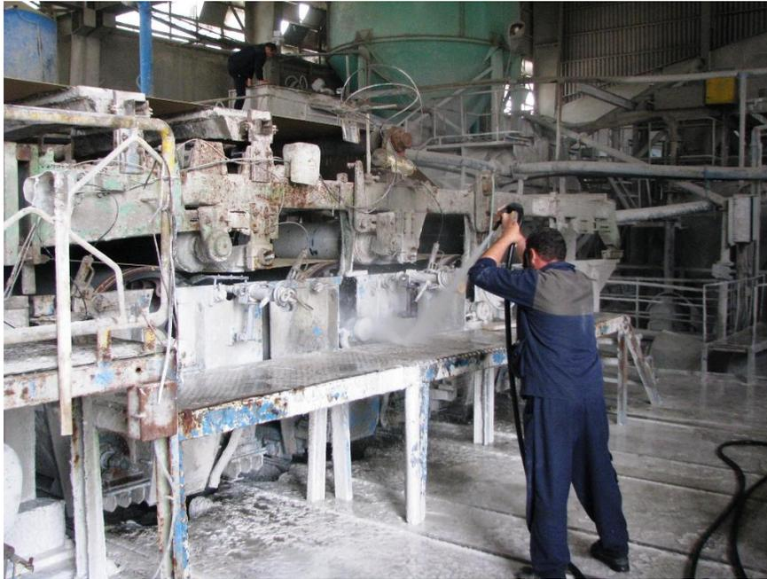
Figure 6-4 Washing the Hatschek machine to remove all remaining asbestos fibres before producing non-asbestos cement board
