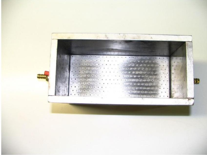
Figure 4-5 Rectangular prismatic aluminium mould for making the specimens in the laboratory
