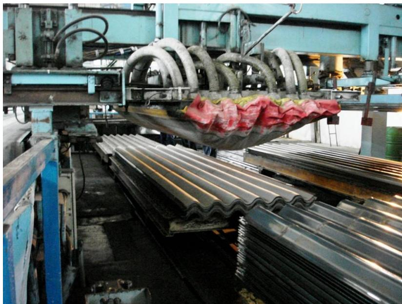
Figure 6-9 Corrugation of sheets by adjusting the moisture content
