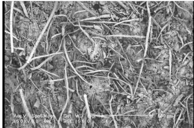
Figure 5-42 Uniform distribution of acrylic and kraft pulp fibres in cement matrix
