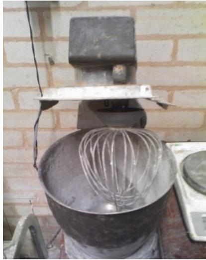
Figure 4-10 Mixing all ingredients in a Hobart mixer with whisk blade
