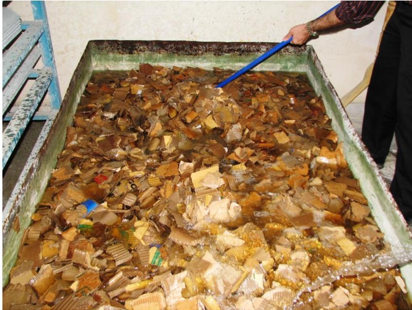
Figure 6-1 Preparation of kraft pulp fibres from shredded cardboard
