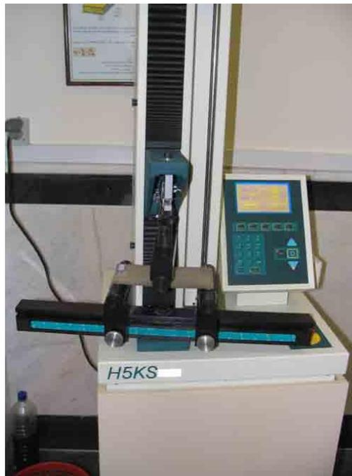
Figure 4-12 Flexural strength test for FCB according to BS EN 12467:2004
