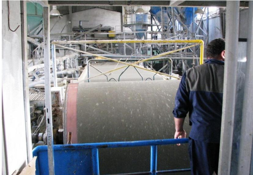
Figure 6-6 Layers built up by winding on the cylinder (mandrel), until the required thickness was obtained
