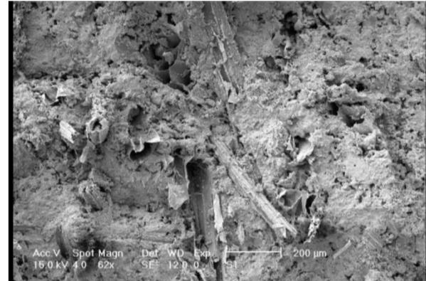
Figure 5-11 Pulling out of eucalyptus fibres from composite
