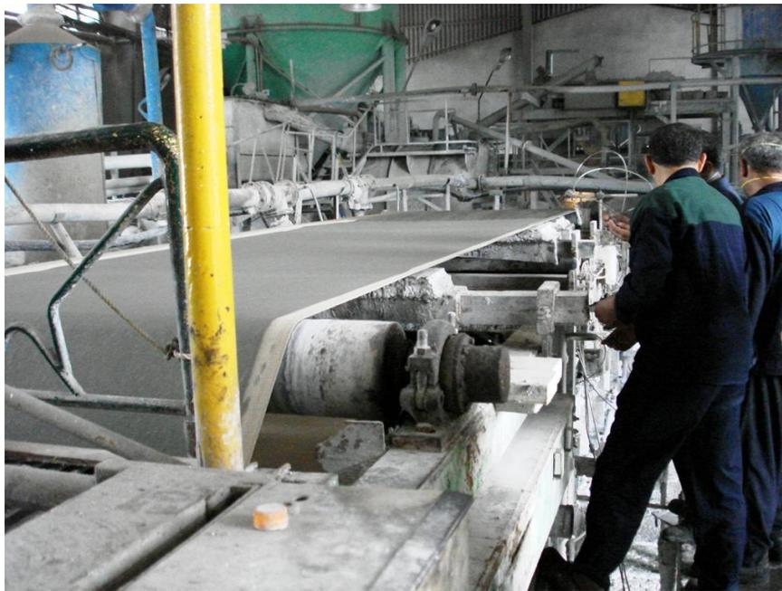
Figure 6-5 Forming the tiny layers on the running felt on the Hatschek machine
