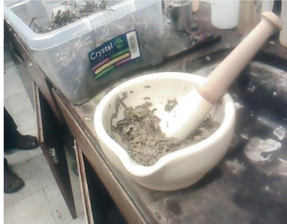
Figure 4-8 Beating fibres in order to refine the natural fibres with pestle and mortar
