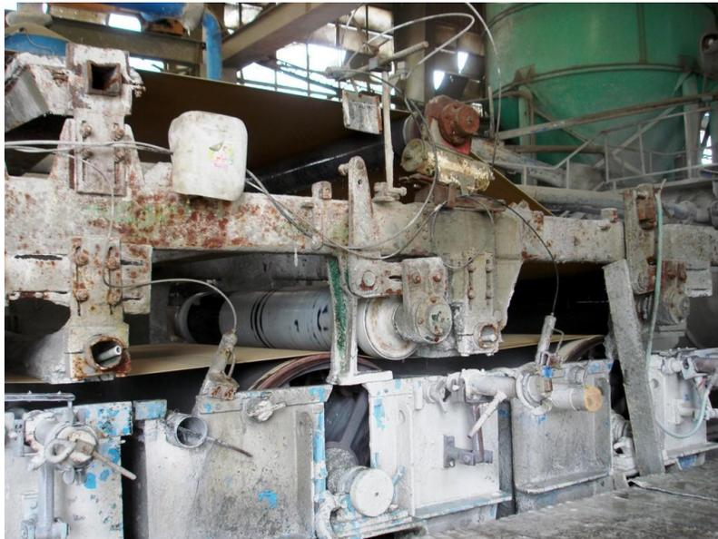
Figure 4-2 Photograph of sieve cylinder in contact with conveyor belt
