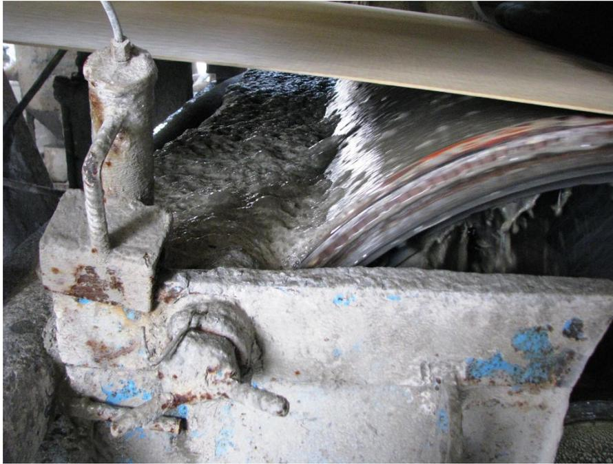
Figure 6-7 Bubble forming in the vat due to cellulose fibres after making several trial cement boards
