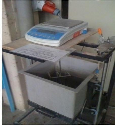
Figure 4-13 System to determine the density of fibre cement board
