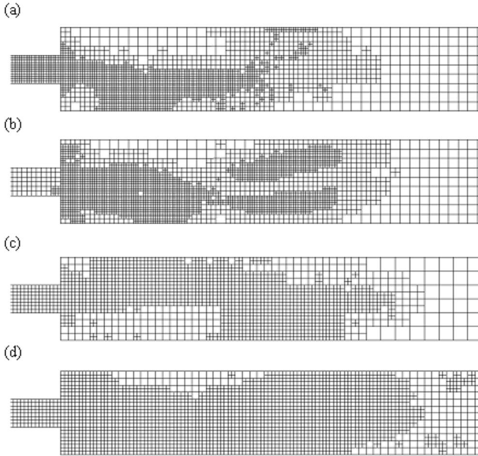
**Figure 3-10 Mesh distribution after gradient adaptation of (a) Static pressure with Initial mesh-1, (b) Y-velocity with Initial mesh-1, (c) Static Pressure with Initial mesh-2 and (d) Y-velocity with Initial mesh-2.**
