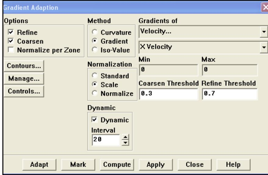
**Figure 3-1 The Gradient Adaption panel in FLUENT.**
