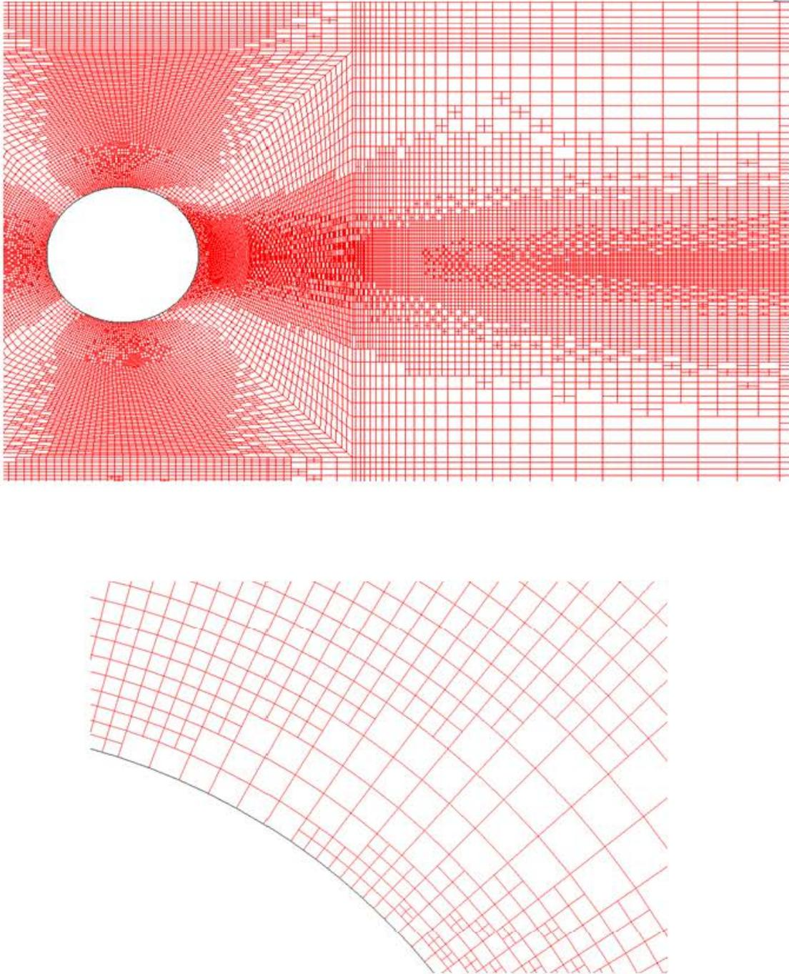
**Figure 5-31 Final mesh distribution for SAG application with  $C^* = 3$  (above) and its near wall region (below).**
