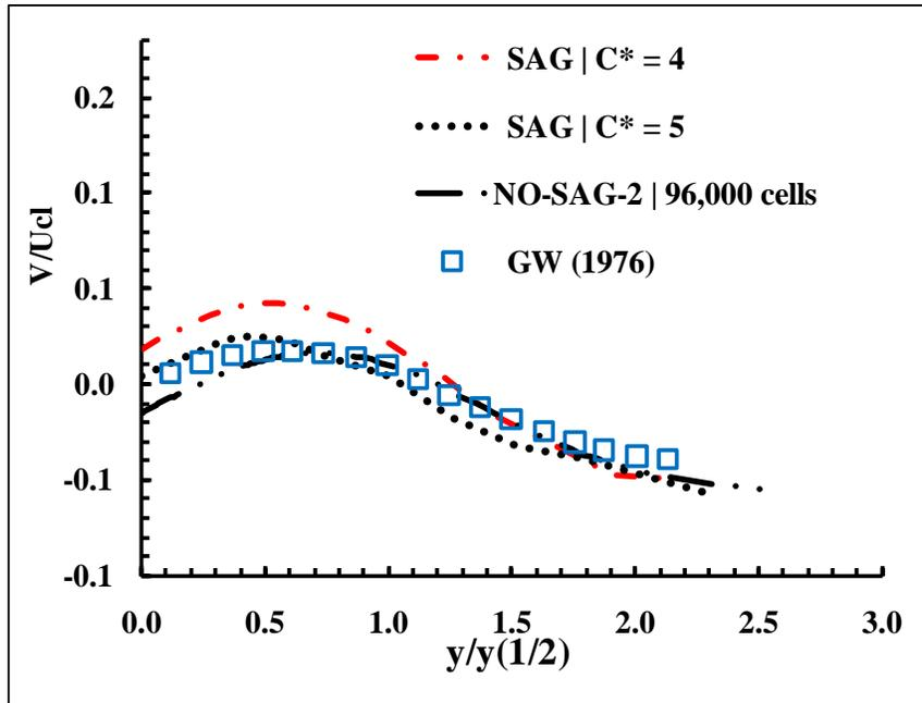
Figure 5-19 Normalized transverse velocity along  $x = 11D$  ; Note: GW = Gutmark & Wygnanski (1976).
