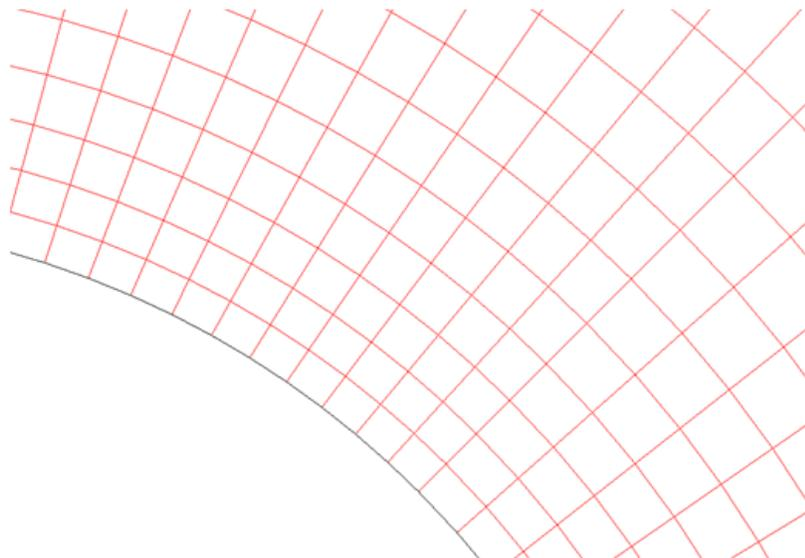
**Figure 5-30 Initial mesh, together with its mesh density near to the cylinder surface, to be used with SAG application.**
