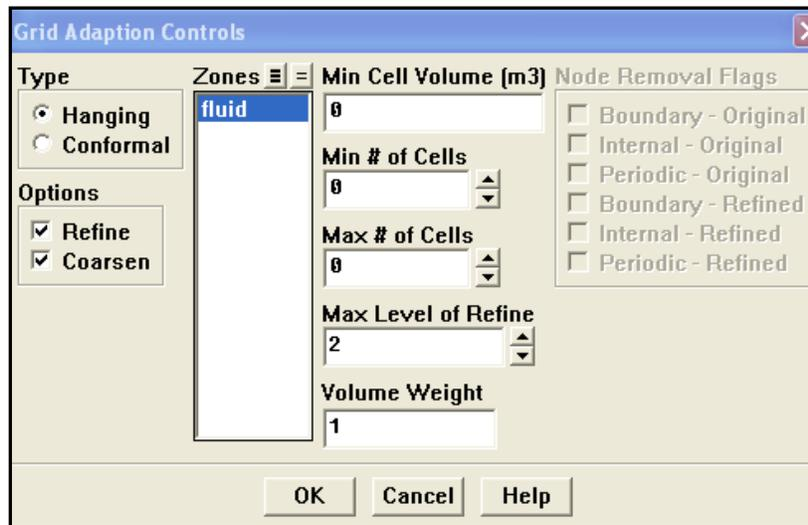
**Figure 3-2 The Grid Adaptation Controls panel in FLUENT.**
