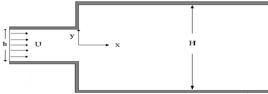
**Figure 3-6 Channel with symmetric sudden expansion geometry.**
