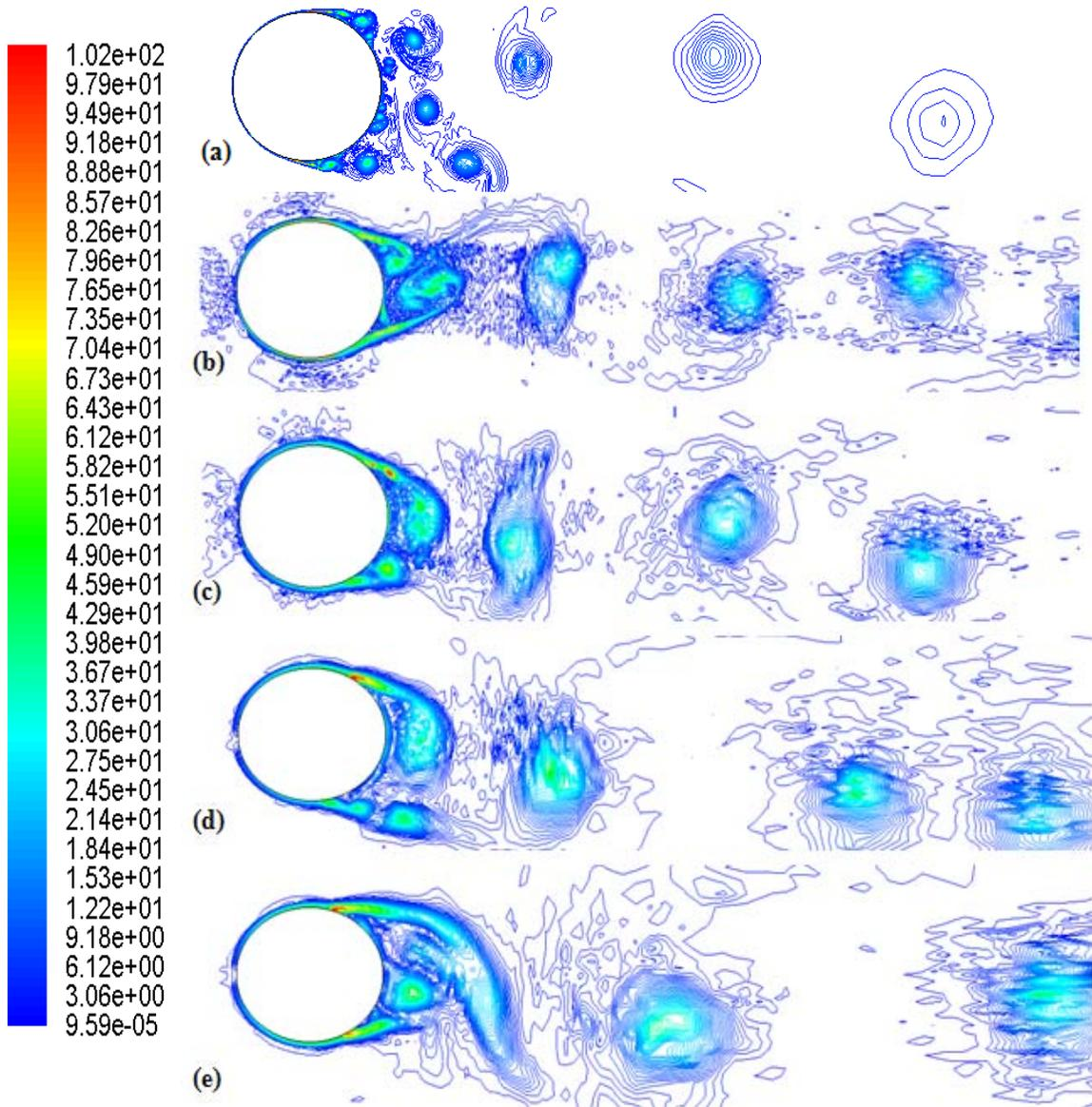
**Figure 5-35 Snap shot of predicted vorticity magnitude, demonstrating vortices formed behind a circular cylinder provided from different test cases; a) NO-SAG-4, b) SAG |  $C^*=3$ , c) SAG |  $C^*=5$ , d) SAG |  $C^*=8$  and e) SAG |  $C^* = 10$ .**
