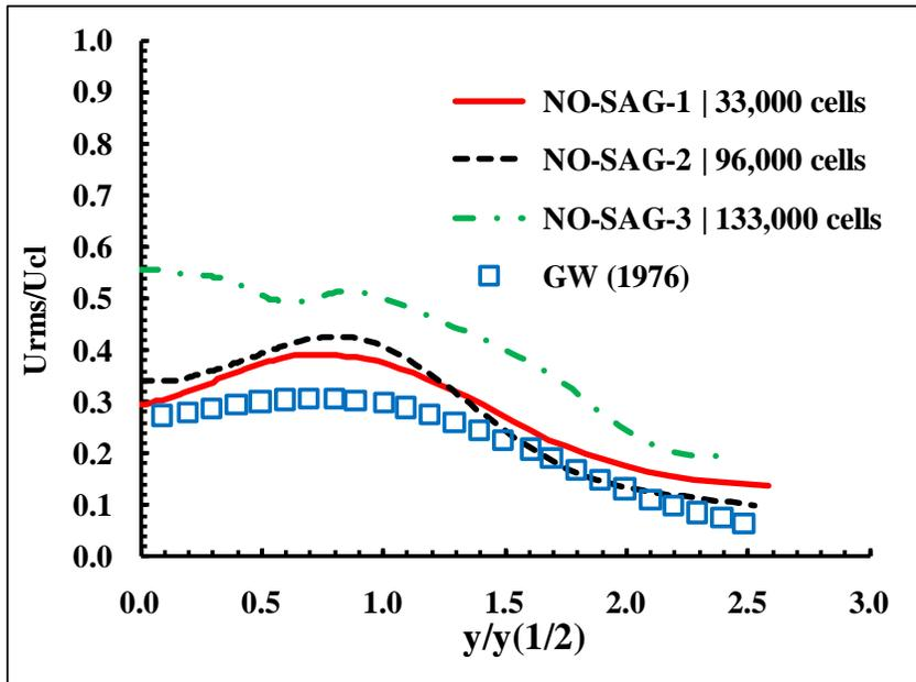
Figure 5-21 Streamwise fluctuation along  $x = 11D$ . Note: GW = Gutmark & Wagnanski (1976).
