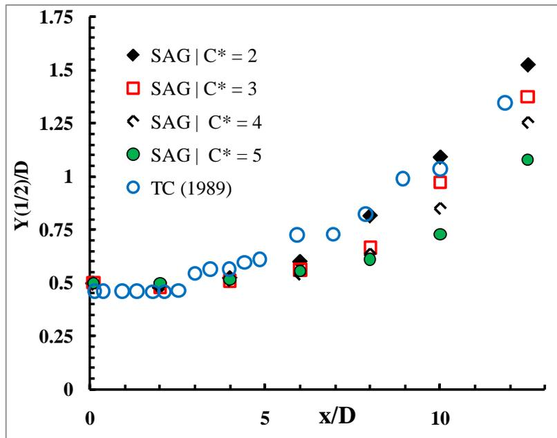
Figure 5-16 Downstream jet half-width growth  $y_{1/2}$ ; values obtained from SAG with different refinement constants compared against the corresponding experimental data. Note: TC = Thomas & Chu (1989).
