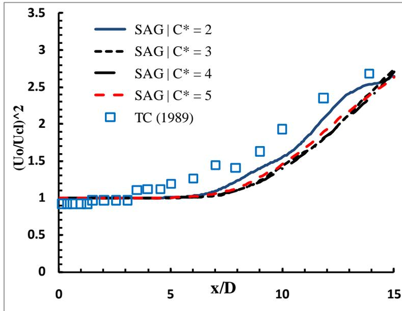
**Figure 5-14 Centreline inverse square of the jet velocity; values obtained from SAG with different refinement constants compared against the corresponding experimental data. Note: TC = Thomas & Chu (1989).**
