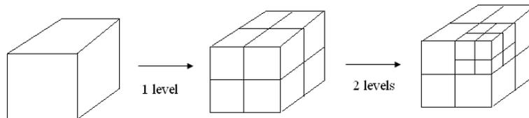
**Figure 2-5 General feature of different levels of refinement for h-refinement approach.**
