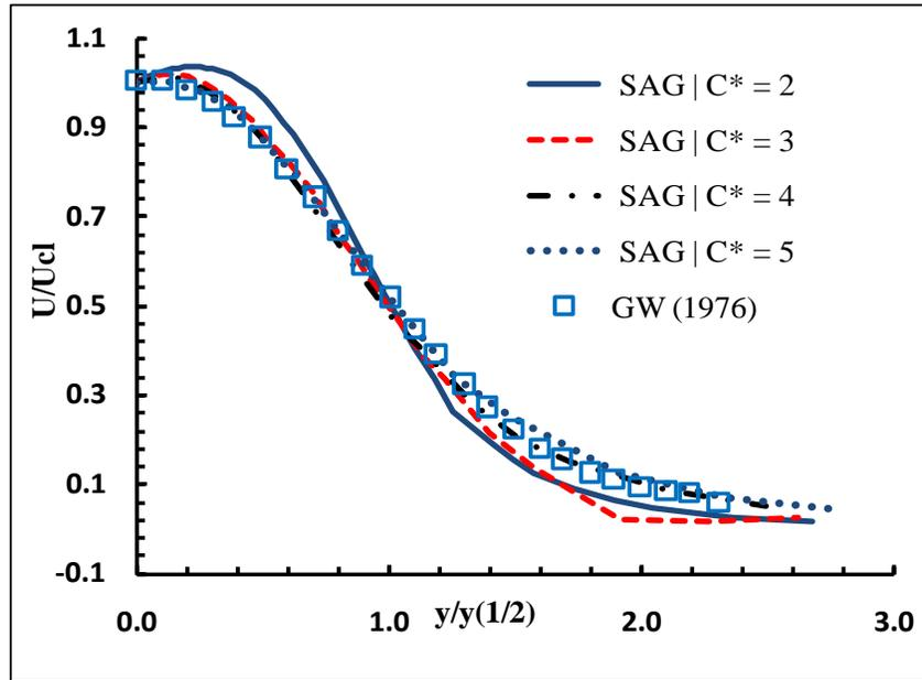
**Figure 5-13 Normalized longitudinal velocities along = 11D ; values obtained from SAG with different refinement constants compared against the corresponding experimental data. Note: GW = Gutmark & Wygnanski (1976).**
