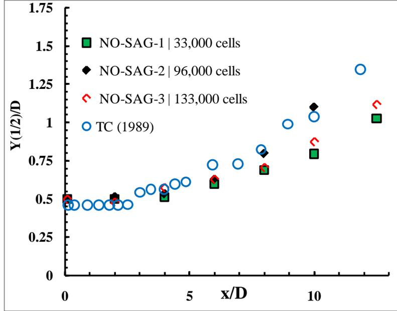
**Figure 5-17 Downstream jet half-width growth  $y_{\frac{1}{2}}$  ; values obtained from the conventional mesh cases compared against the corresponding experimental data. Note: TC = Thomas & Chu (1989).**
