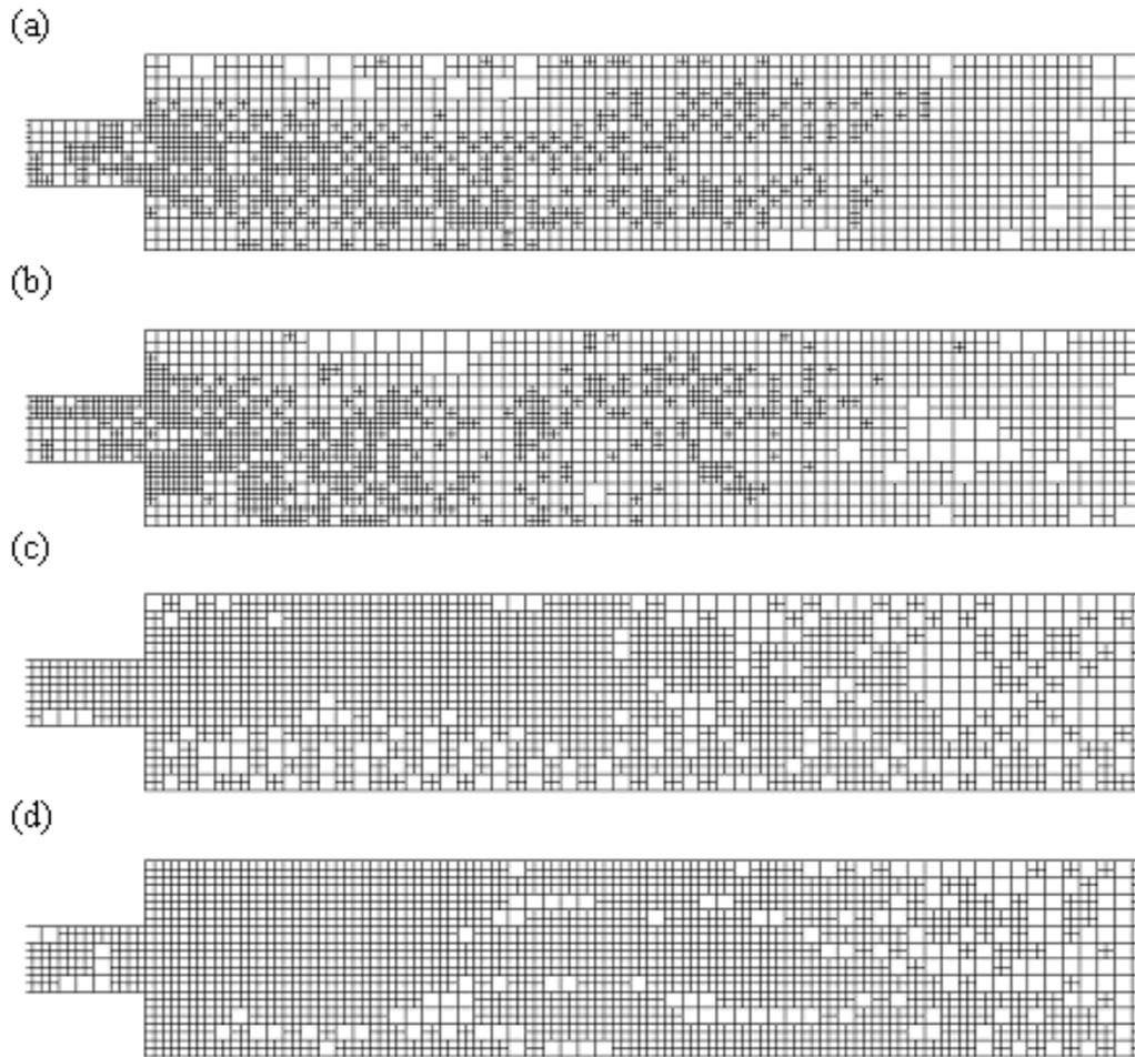
**Figure 3-11 Mesh distribution after curvature adaptation of (a) Static pressure with Initial mesh-1, (b) Y-velocity with Initial mesh-1, (c) Static Pressure with Initial mesh-2 and (d) Y-velocity with Initial mesh-2.**
