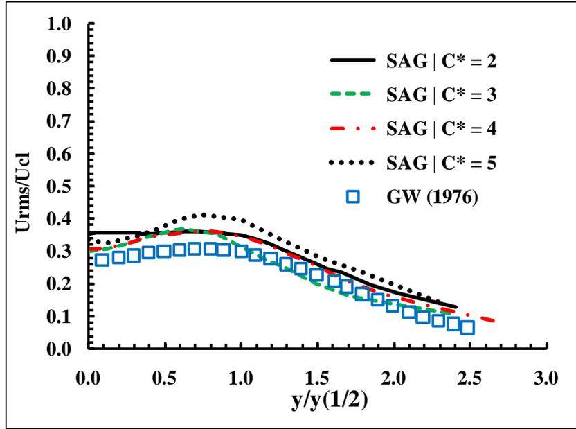
Figure 5-20 Streamwise fluctuation along  $x = 11D$ . Note: GW = Gutmark & Wagnanski (1976).
