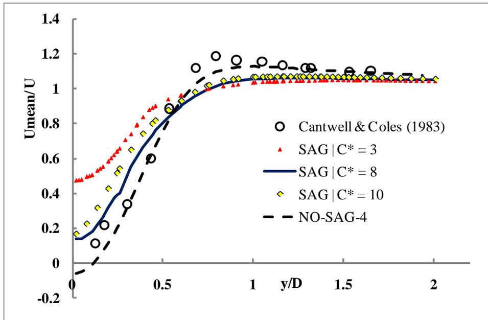
**Figure 5-37 Time-averaged X-velocity distribution along the line  $x = D$  of the cylinder for selected cases both those from conventional mesh and those from SAG study.**
