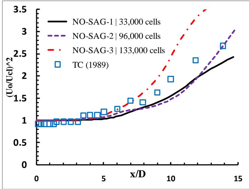
Figure 5-15 Centreline inverse square of the jet velocity; values obtained from the conventional mesh cases compared against the corresponding experimental data. Note: TC = Thomas & Chu (1989).
