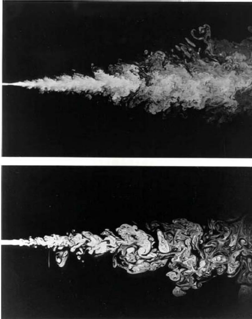
**Figure 5-1** Turbulent jets issued from a round shape orifice at different Reynolds numbers, above)  $Re \approx 10^4$  and below)  $Re \approx 2.5 \times 10^3$  with flow direction from left to right. Data from Dimotakis *et al.* (1983).
