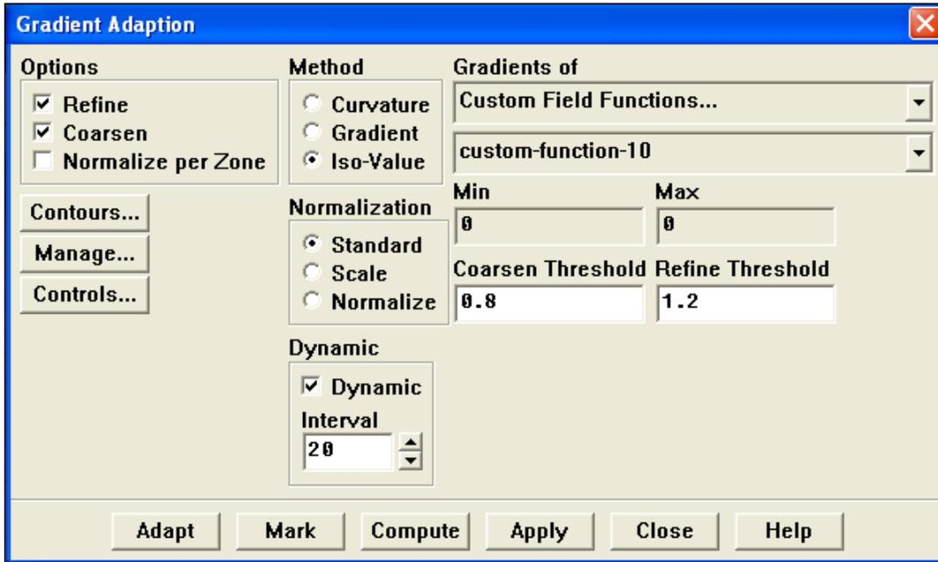
**Figure 4-5** The Gradient Adaption panel in FLUENT with the refinement criterion used for turbulence case studies in Chapter 5.
